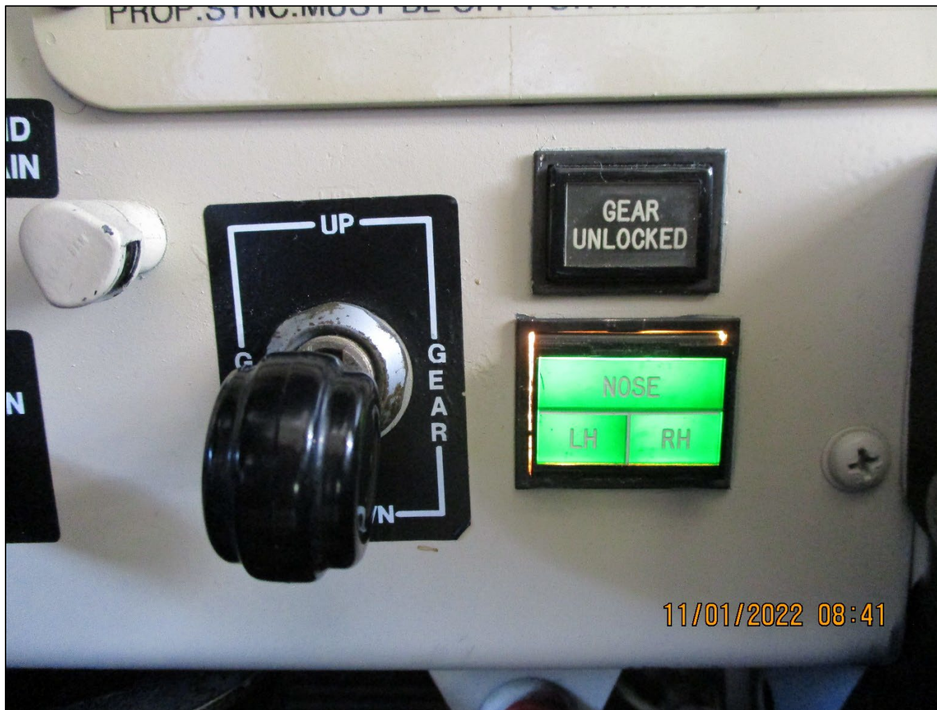
Photograph 5 - View of the landing gear indicator lights displaying all three gear down and locked postaccident (Photo Courtesy of FAA)
