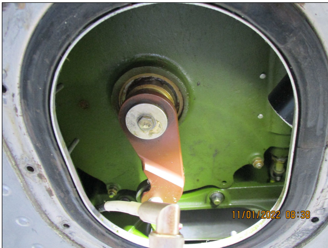
Photograph 4 - Landing gear actuator arm (Photo Courtesy of FAA)
