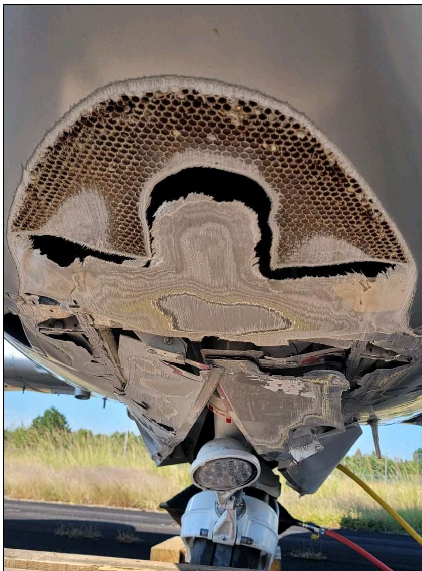
Photograph 2 - Overview of the substantial damage sustained to the fuselage (Photo courtesy of FAA)
