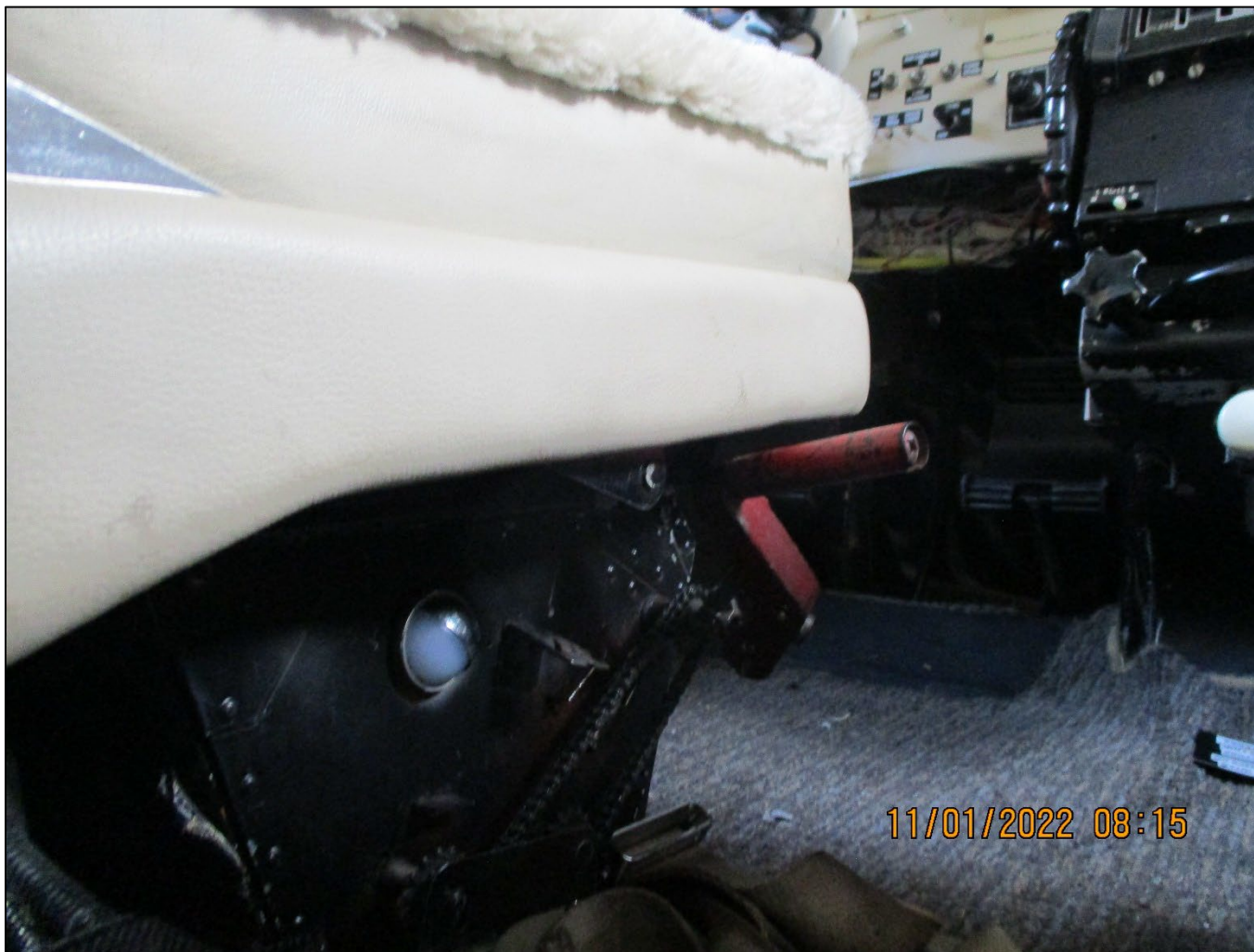
Photograph 6 - View of the landing gear manual hand crank found in an intermediate position (Photo Courtesy of FAA)
