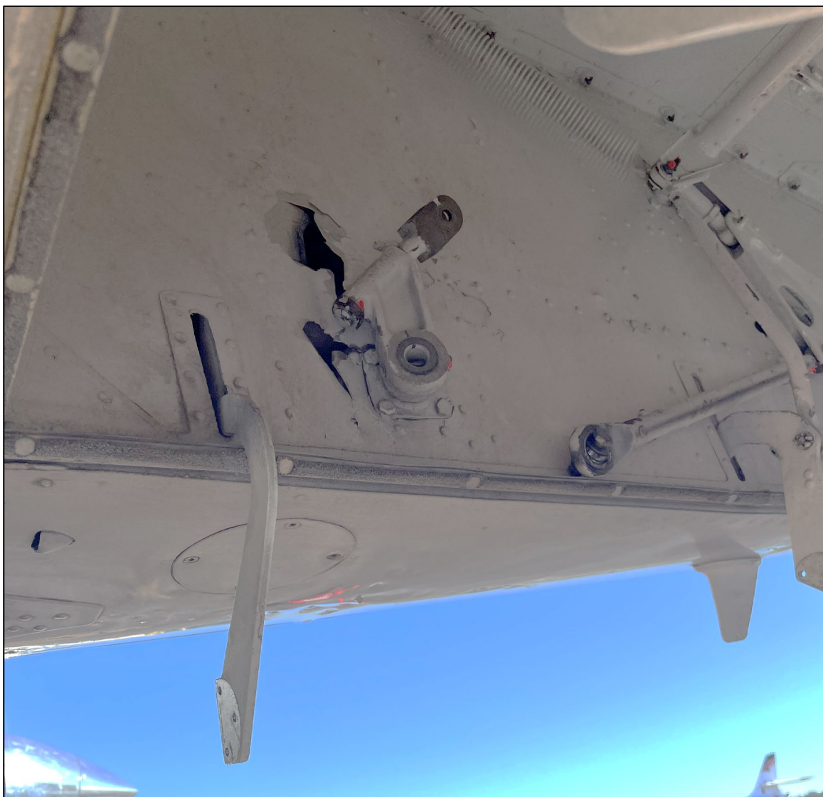
Photograph 3 - View of the disconnected NLG torque tube (reportedly disconnected by maintenance personnel after the accident) (Photo courtesy of FAA)
