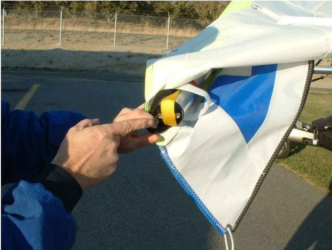
Figure 1: View Showing How Sail Strap Is Positioned over Leading Edge Tube Trim Tip Cap.
