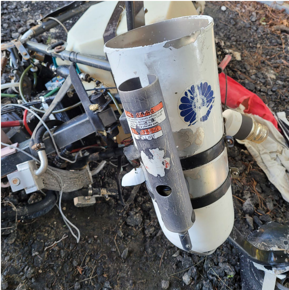
Figure 7: View of the Airframe Ballistic Parachute Components.
