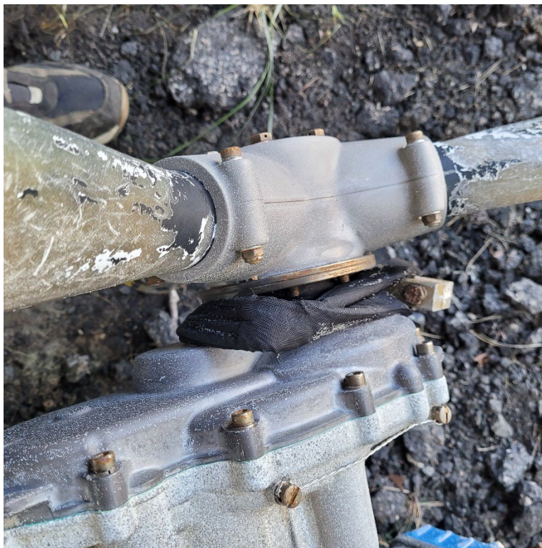
Photo 9: View Showing the Airframe Ballistic Parachute Webbing Between Propeller and Engine.
