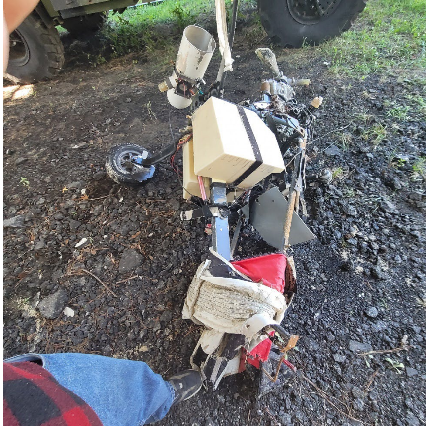
Figure 11: View Showing the Fuel Tank Secured by One Strap.
