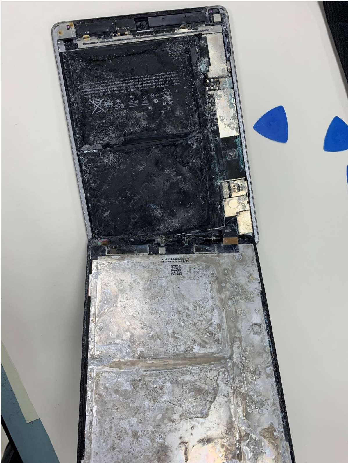
Figure 4. Heavily corroded motherboard inside the Apple iPad Air 2 as received.
