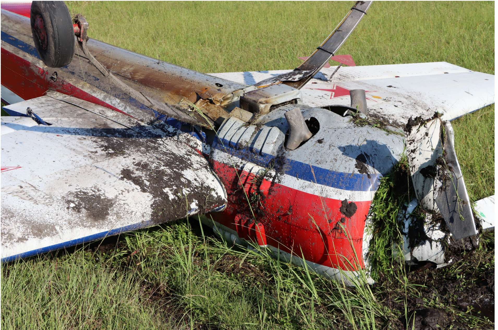
Photo 3 - Digital Photograph Provided by Alachua County Sheriff's Office. Left Forward Quartering View of the Inverted Airplane At the Accident Site. Note the Structural Damage (Buckling) of the Lower Fuselage near the Left Main Landing Gear Attach Point.
