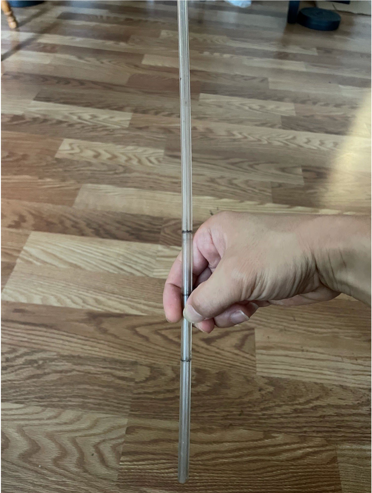
Figure 2: Digital Photograph Provide by Pilot. View Depicting the Level in Both Fuel Tanks During the Pilot's Preflight Inspection.
