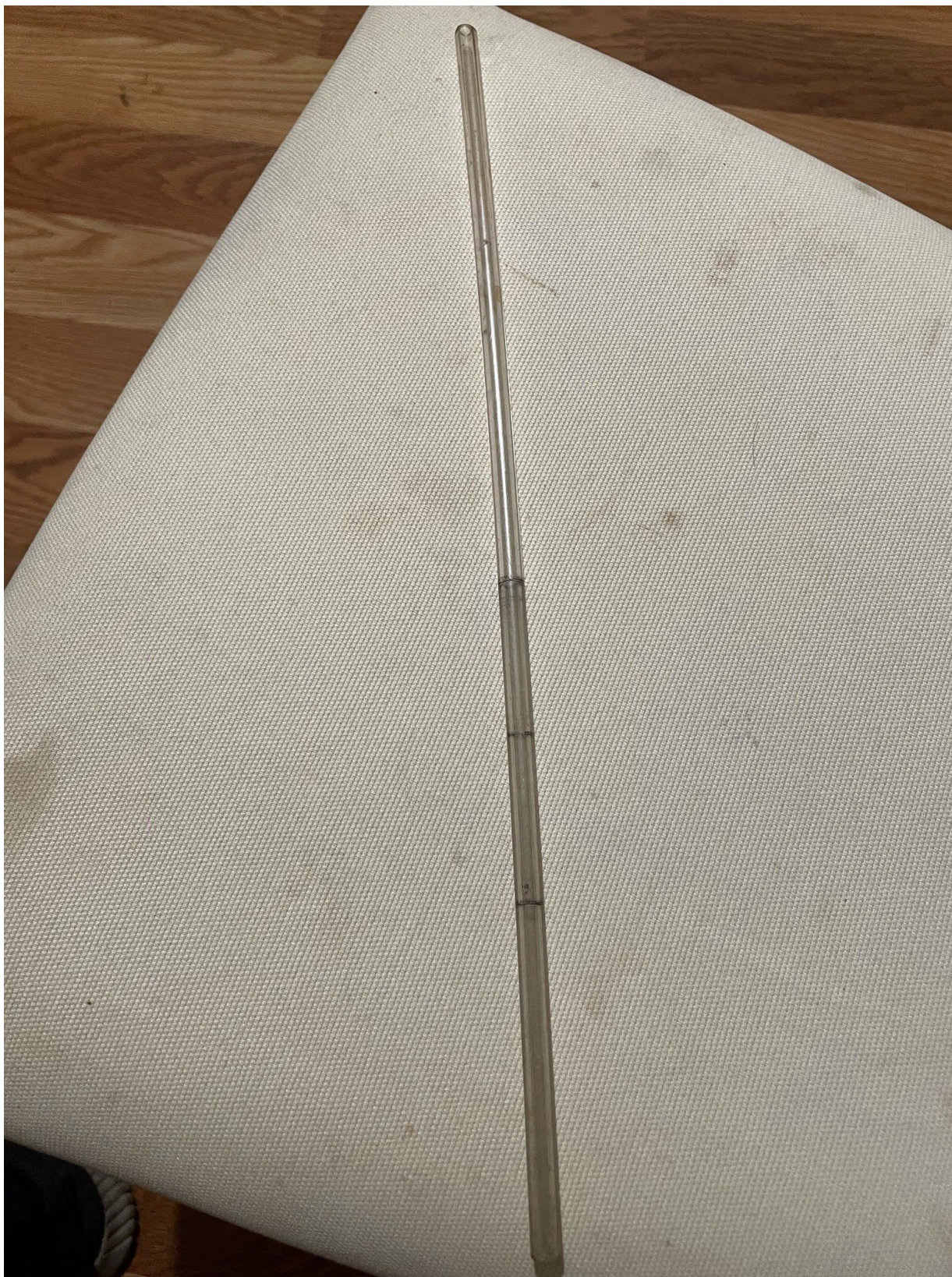
Figure 1: Digital Photograph Provide by Pilot. View of the Dipstick Used by the Pilot During His Preflight Inspection.
