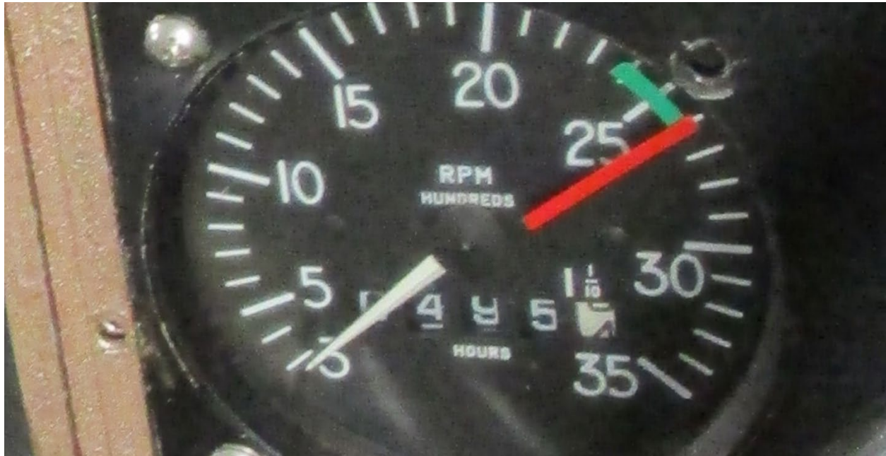
Figure 1: FAA Digital Photograph. View of the Tachometer Taken Postaccident. Reading 495.4
