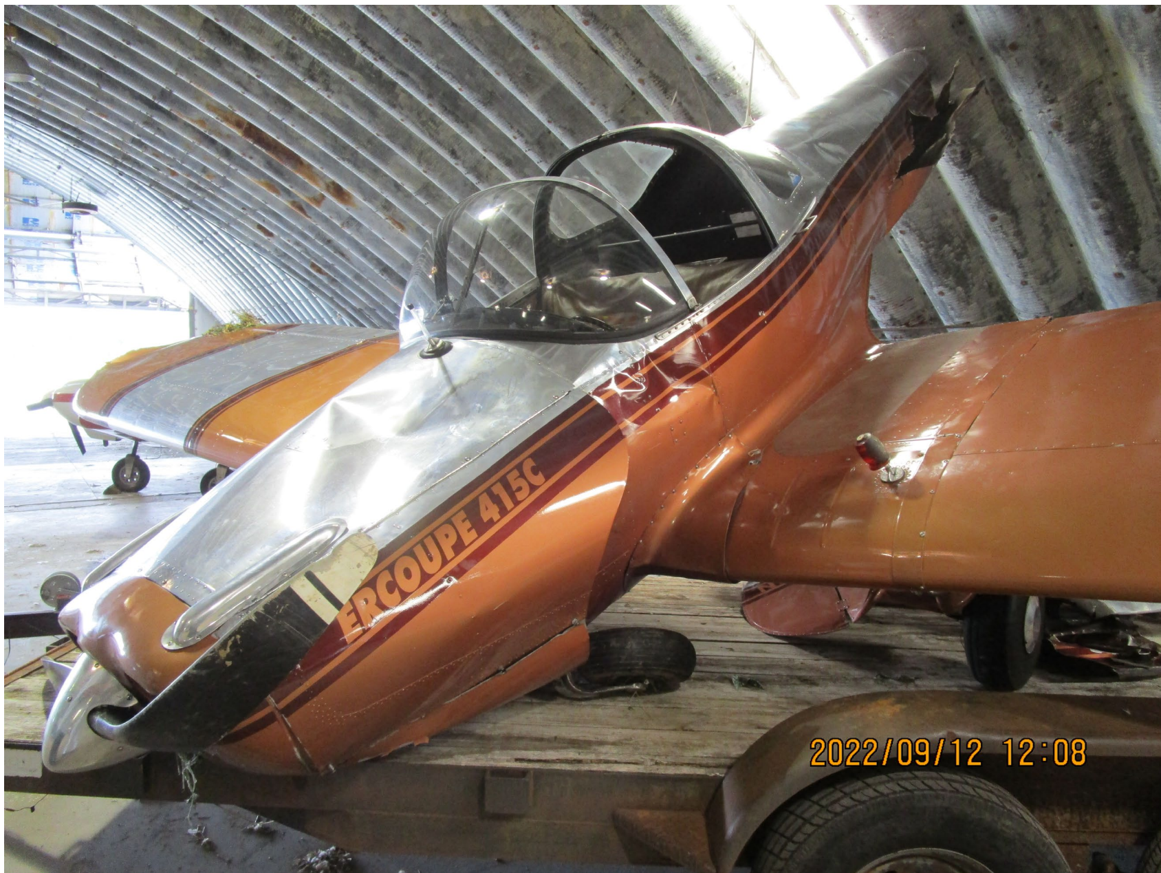
Photo 1 – FAA Digital Photograph. Left Forward Quartering View of the Airplane Following Recovery. Note the Separated Aft Empennage.
