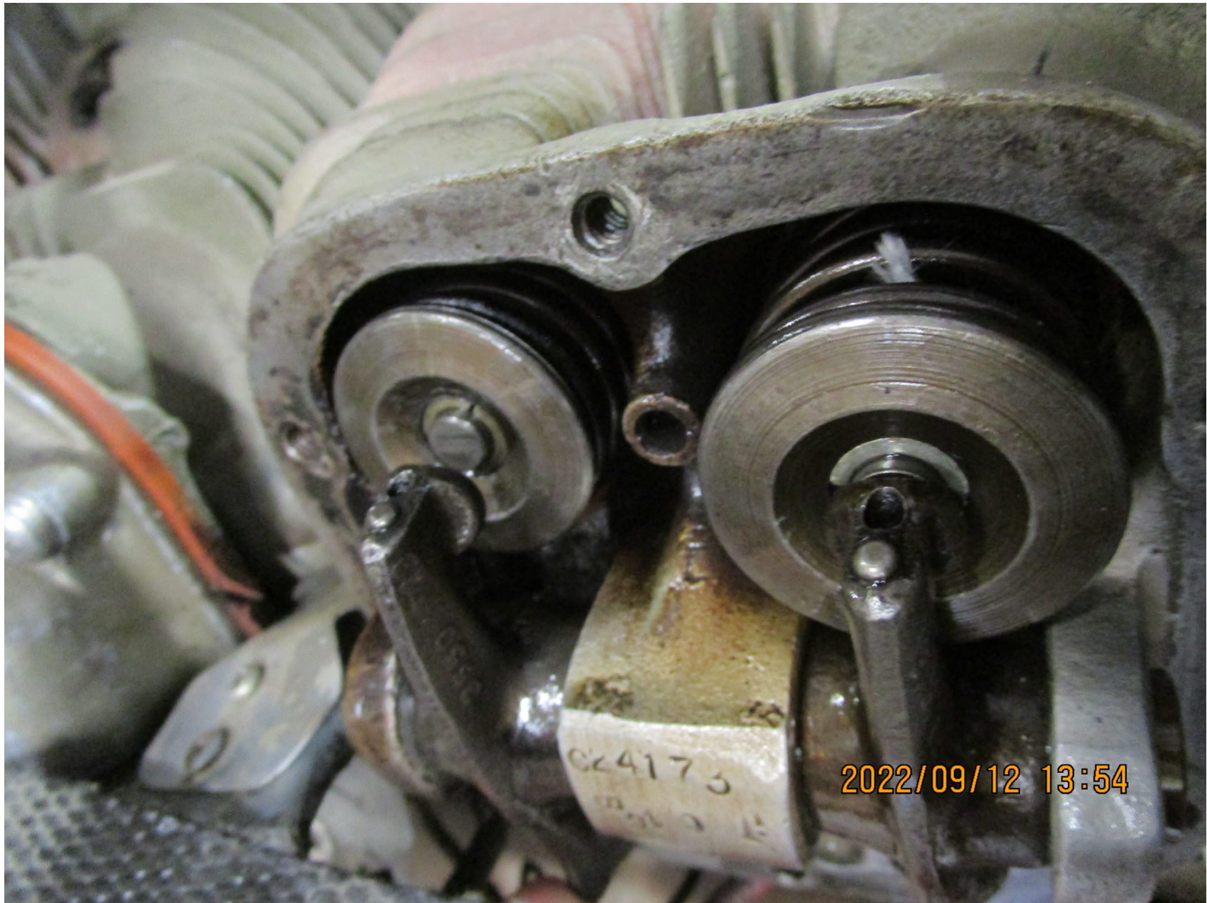
Photo 3 - FAA Digital Photograph. View Showing the Open Exhaust Valve of the No. 2 Cylinder.
