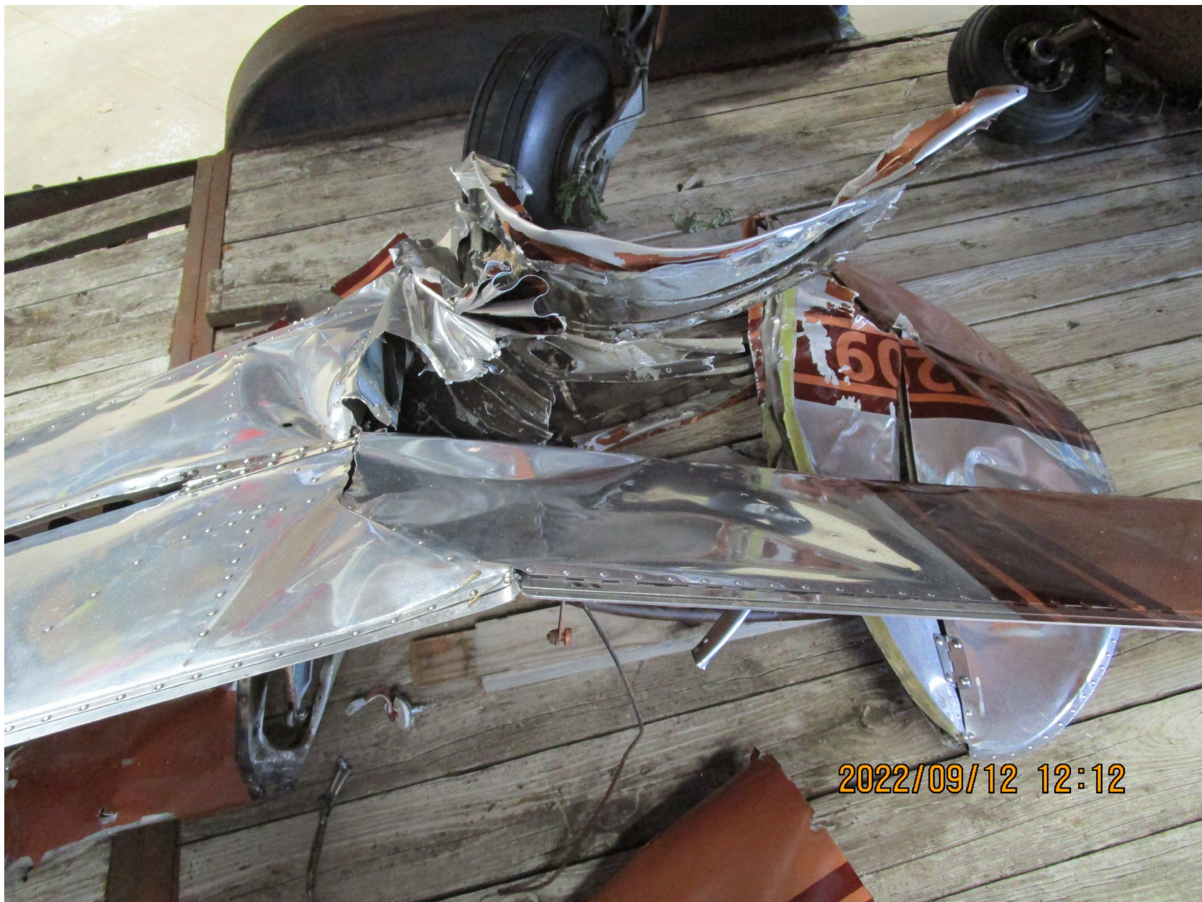
Photo 2 – FAA Digital Photograph. View of the Structurally Damaged Aft Empennage.
