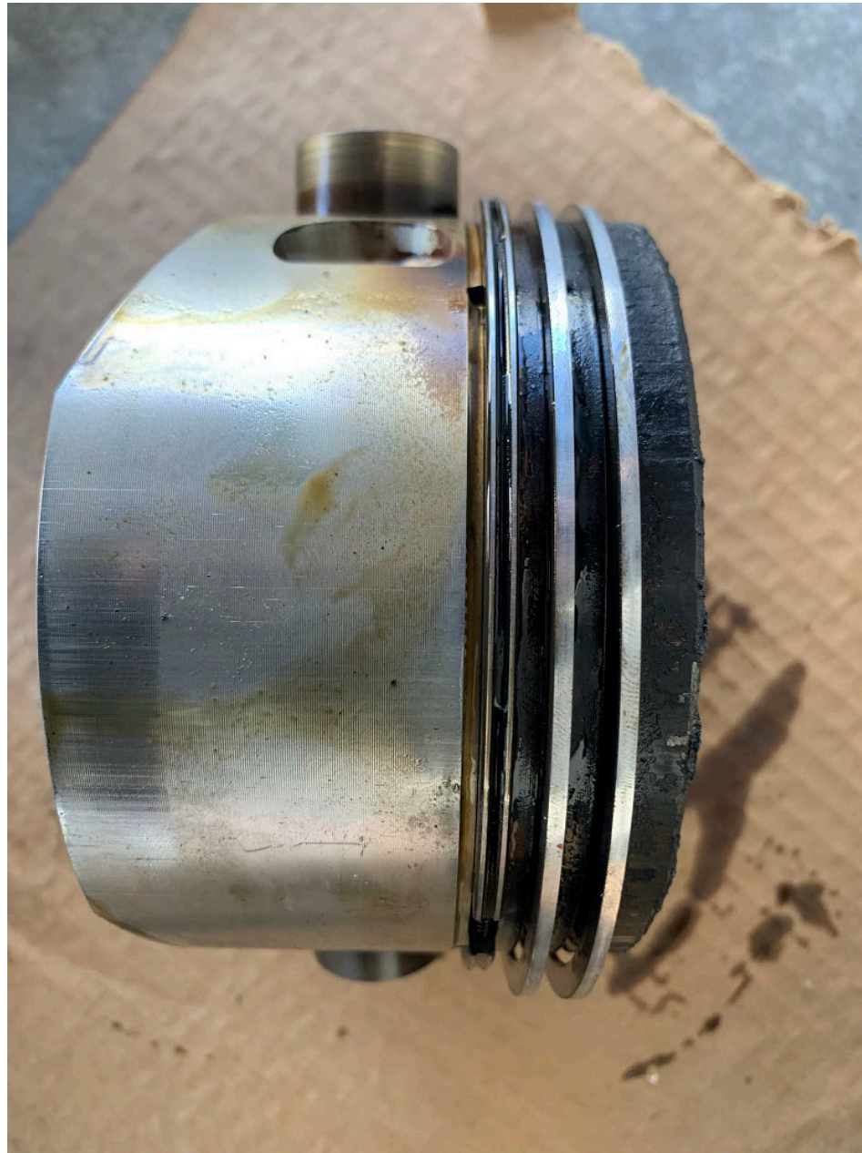
Photo 4 – View of No. 1 Piston Skirt (Photo Courtesy of FAA)
