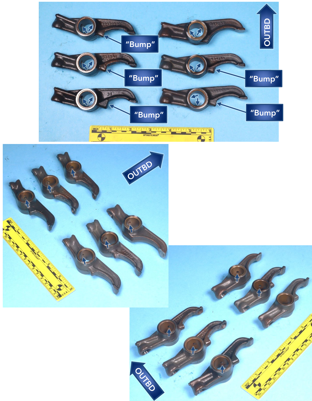
Figure 16. Views of the exhaust rocker arms. Unlabeled arrows point to locations of oil passage holes in the rocker bushings.
