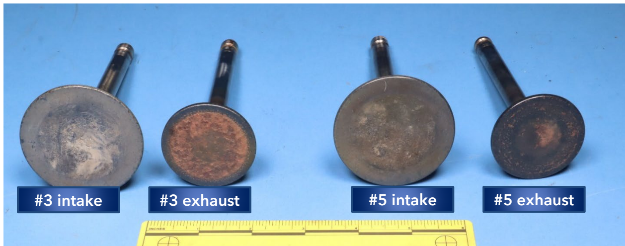
Figure 8. Valve head faces from the number 3 and number 5 cylinders.
