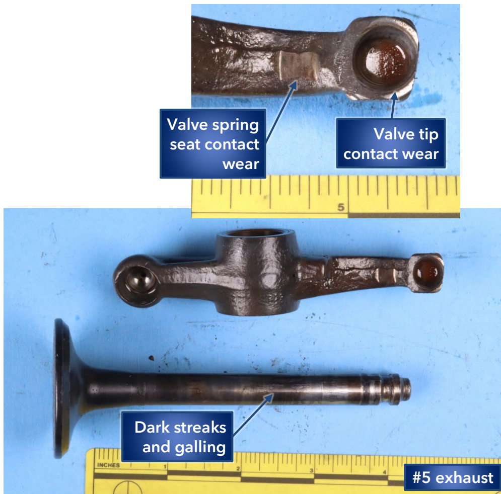
Figure 11. Overall view of the number 5 cylinder exhaust valve and rocker arm (lower image) with a closer view of the valve contact pad on the rocker arm (upper image).
