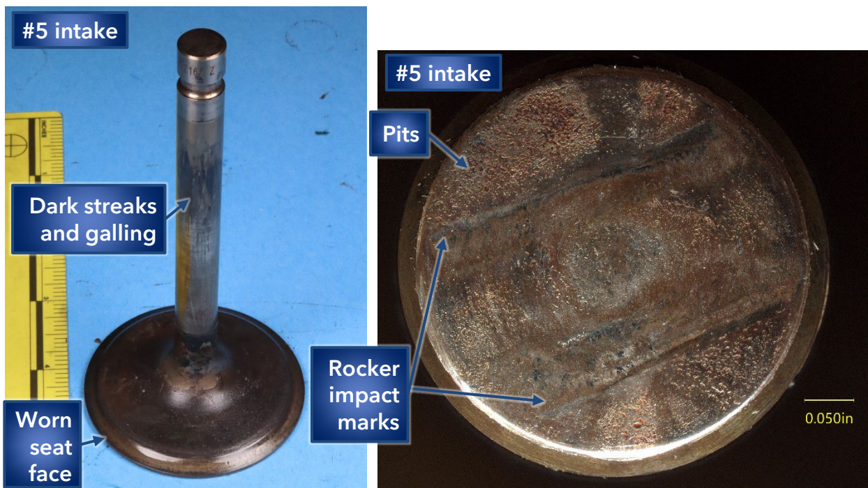
Figure 9. Overall view of the number 5 cylinder intake valve (left image) with a closer view of the tip end face (right image). Longitudinally-oriented dark streaks and galling damage were observed on the stem, and impact marks were observed on the tip end face.
