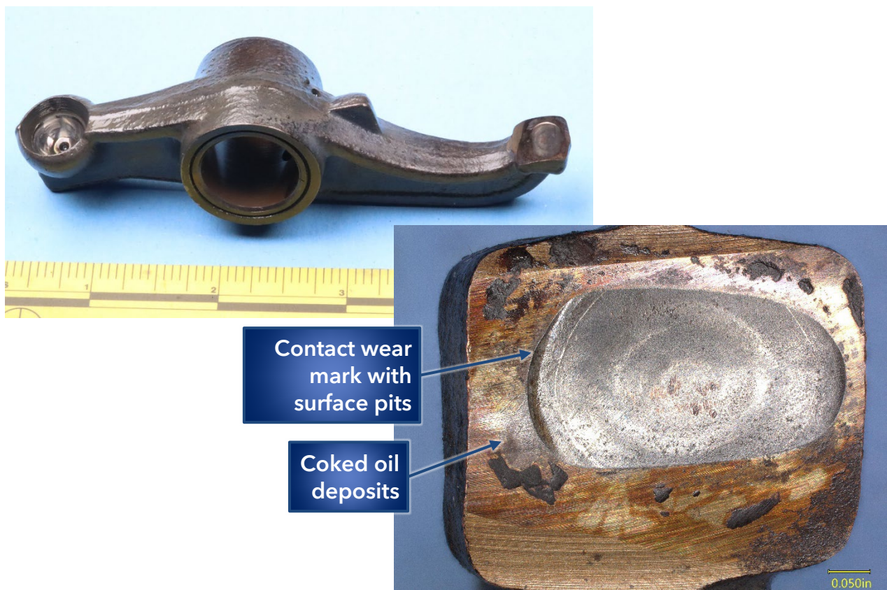
Figure 13. View of an unlabeled exhaust rocker arm (upper image) with a closer view of the valve contact pad (lower image).
