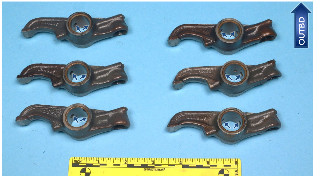
Figure 18. Intake rocker arms with unlabeled arrows pointing to oil passage holes in the bushings.
