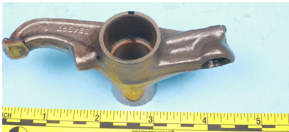
Figure 19. Intake rocker arm with the bushing partially removed. No circumferential oil groove was observed in the rocker bore in 4 of the 6 intake rocker arms including the representative rocker arm shown here.
