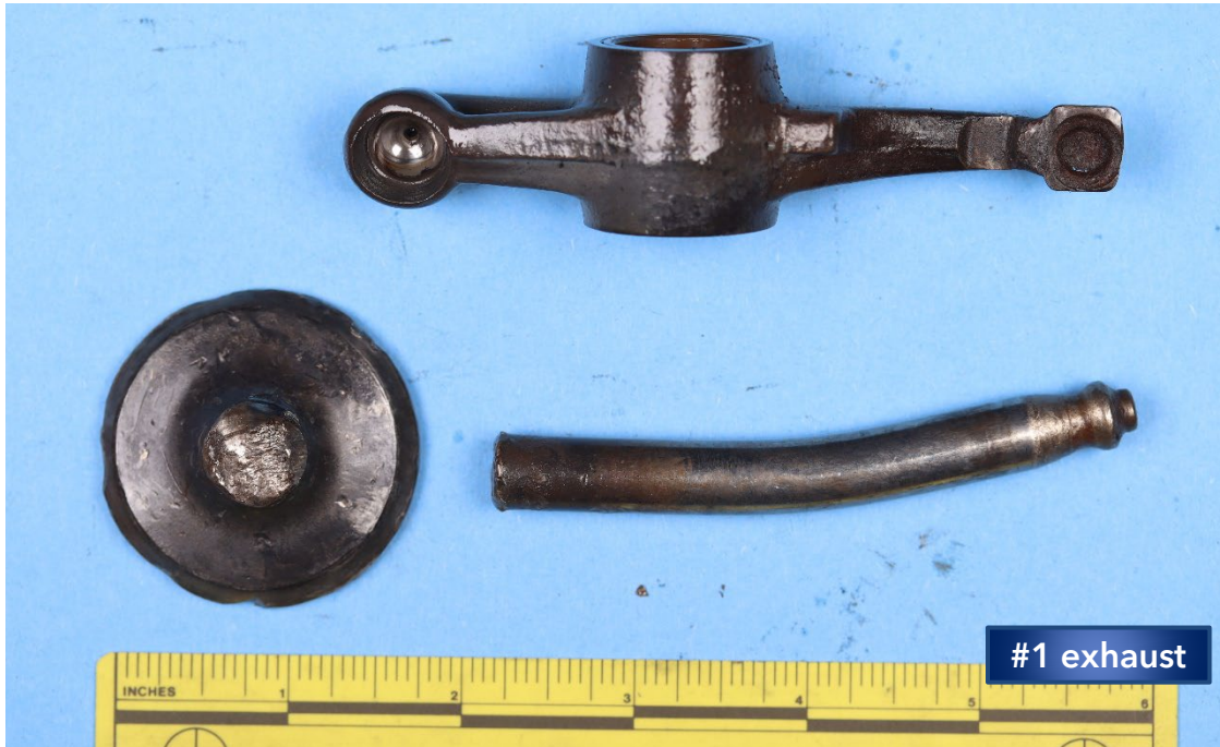
Figure 2. Closer view of the exhaust valve and associated rocker arm from cylinder number 1.
