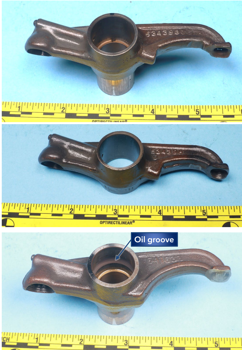
Figure 17. Number 1 exhaust rocker arm (upper image), number 5 exhaust rocker arm (middle image), and unlabeled exhaust rocker arm that did not have a “bump” (lower image) after pressing the bushings from the respective rocker bore. A circumferential oil groove was present in the exhaust rocker arm without a bump as indicated in the lower image, and no oil groove was observed in the rocker bore for other exhaust rocker arms including from the number 1 and number 5 cylinders as shown.
