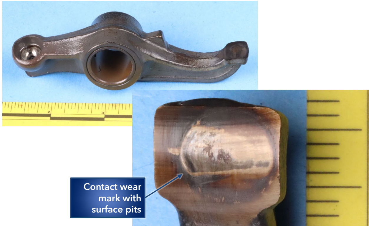
Figure 14. View of an unlabeled exhaust rocker arm (upper image) with a closer view of the valve contact pad (lower image).
