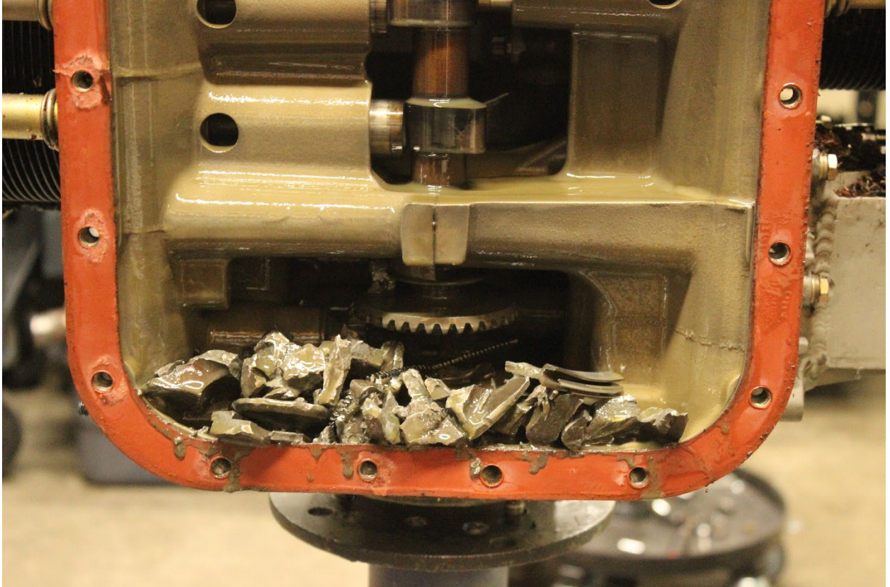
Figure 7 Metal fragments found in the oil sump.
