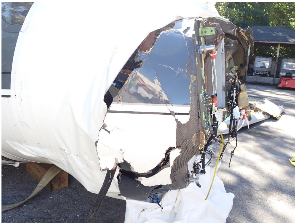
Photo 8: NTSB Digital Photograph. Right Side View of the Front Pressure Bulkhead, and Fuselage Immediately Aft of it.
