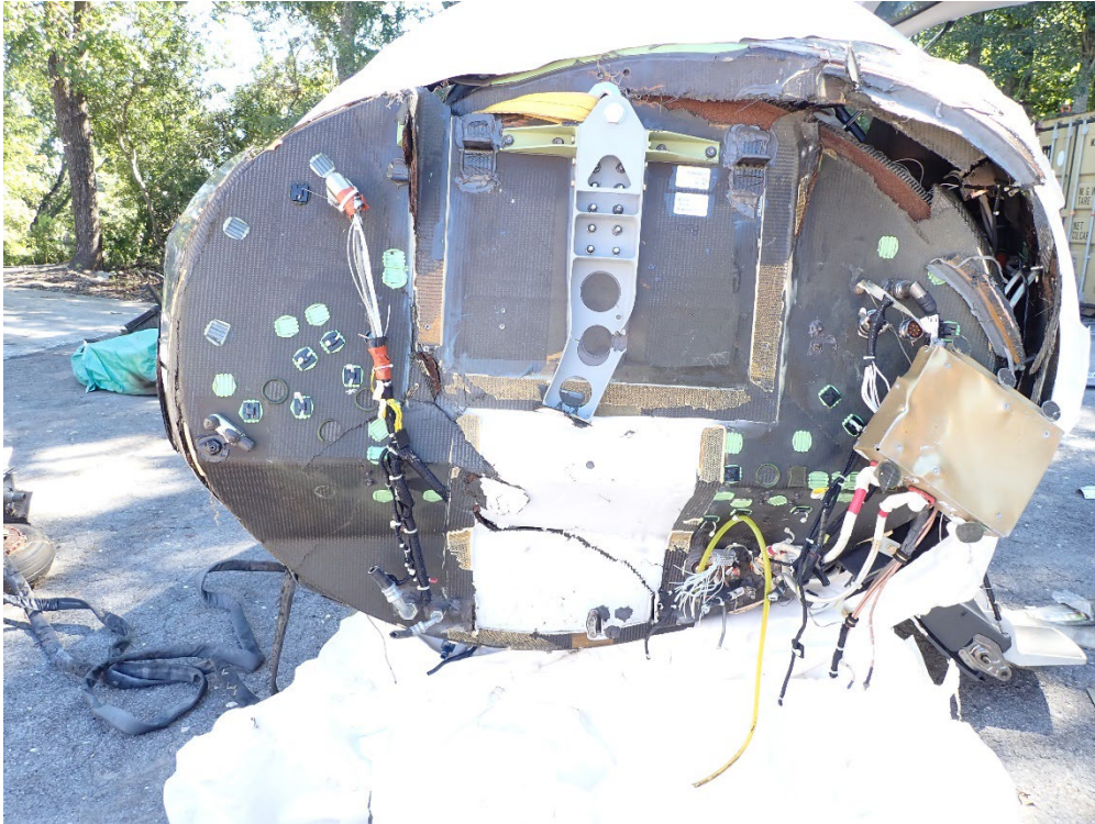
Photo 7: NTSB Digital Photograph. Frontal View Looking Aft to Front Pressure Bulkhead. Note the Extensive damage.
