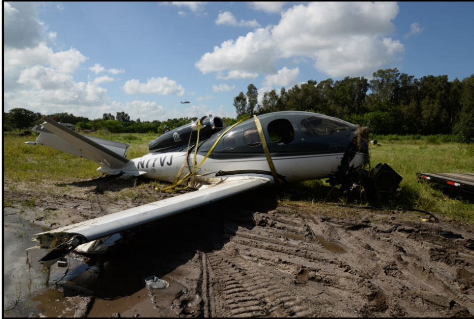
Figure 4: Right Side View of the Airplane After Being Airlifted from the Accident Site.
