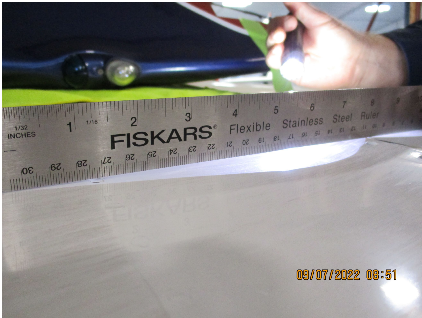
Photo 4 – Damage to Wing
