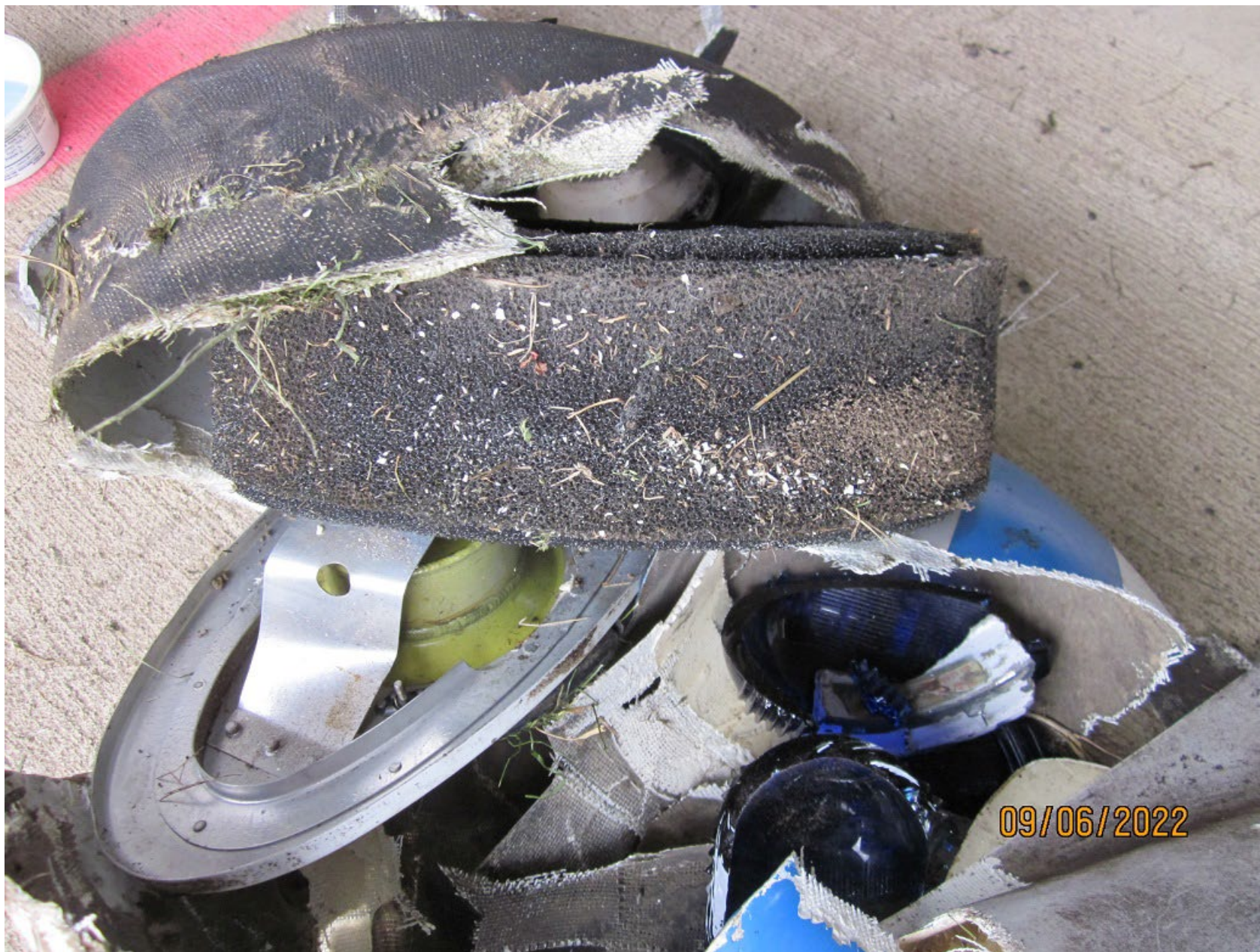
Photo 6 – Air Filter (Photo Courtesy of FAA)
