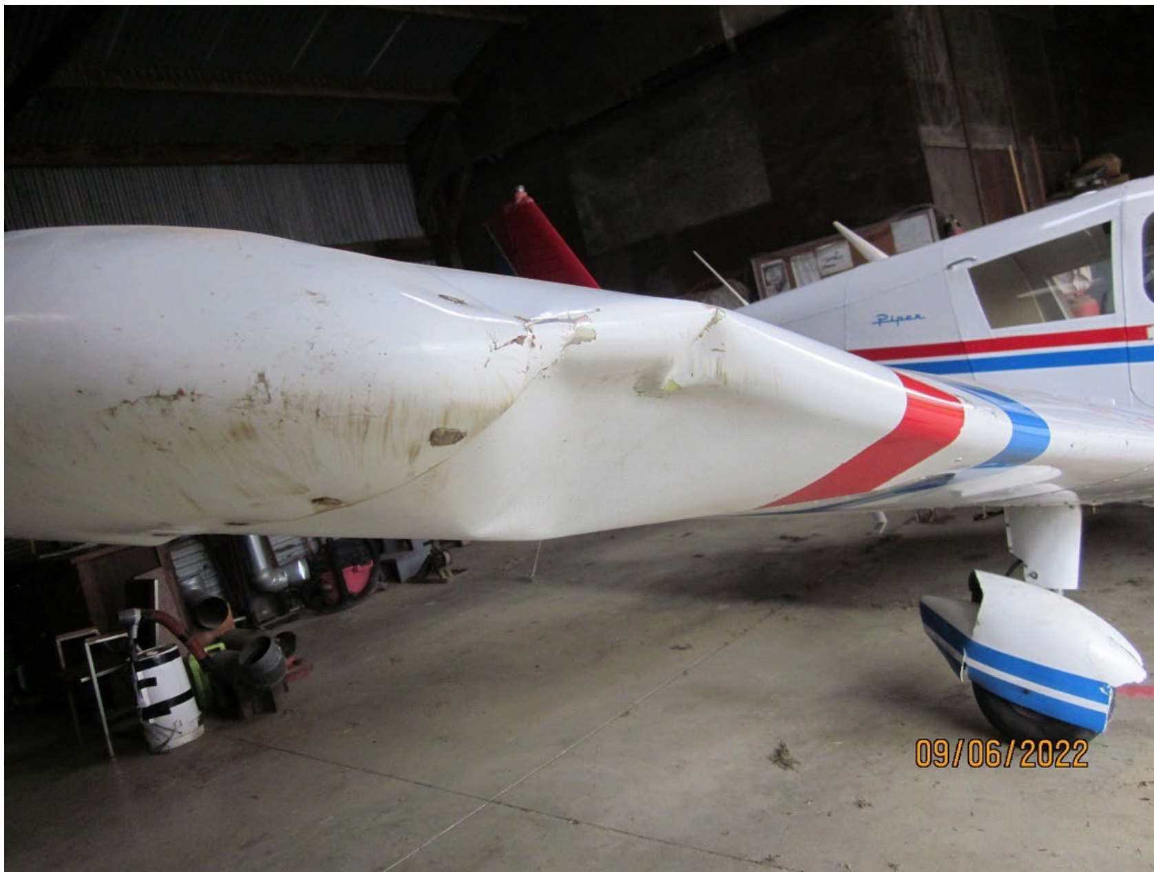
Photo 2 – Right Wing Damage (Photo Courtesy of FAA)
