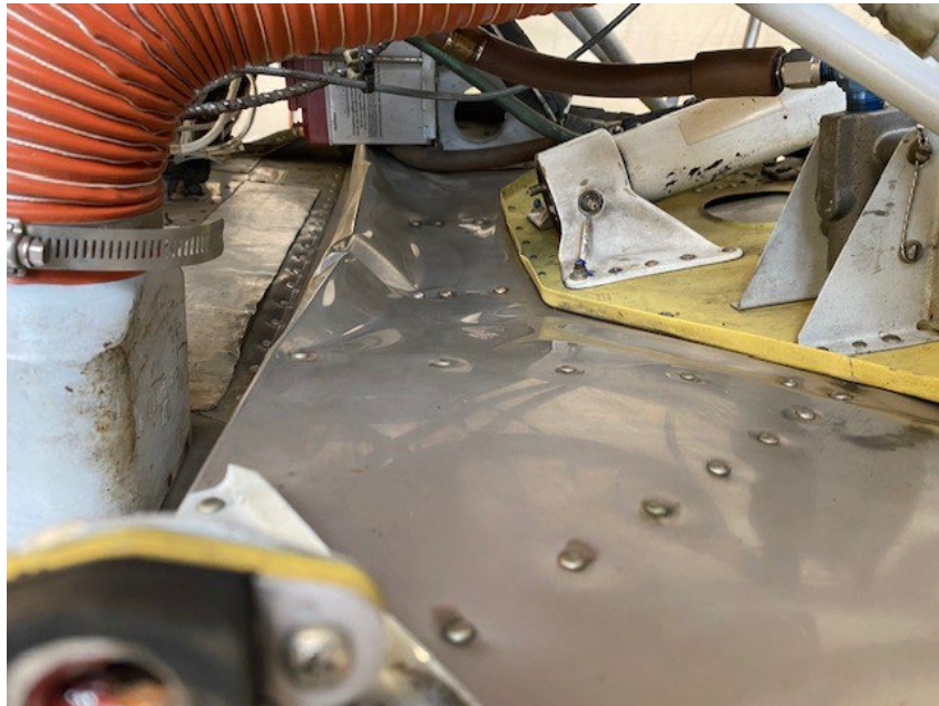
Photos 7, 8, 9: Overview of damage to the firewall (Photo Courtesy of FAA)
