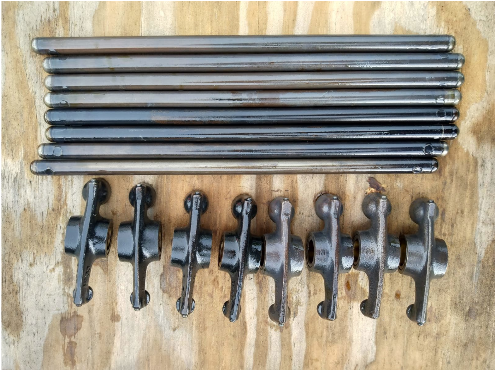
Photo 2 – View of Rocker Arms and Pushrods as Found (FAA)
