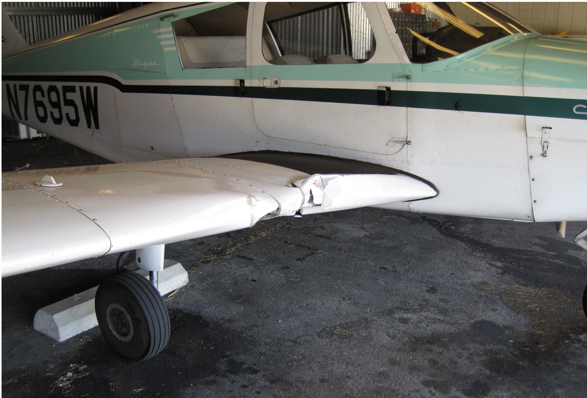
Photo 1 – Right wing leading edge damaged, (FAA)
