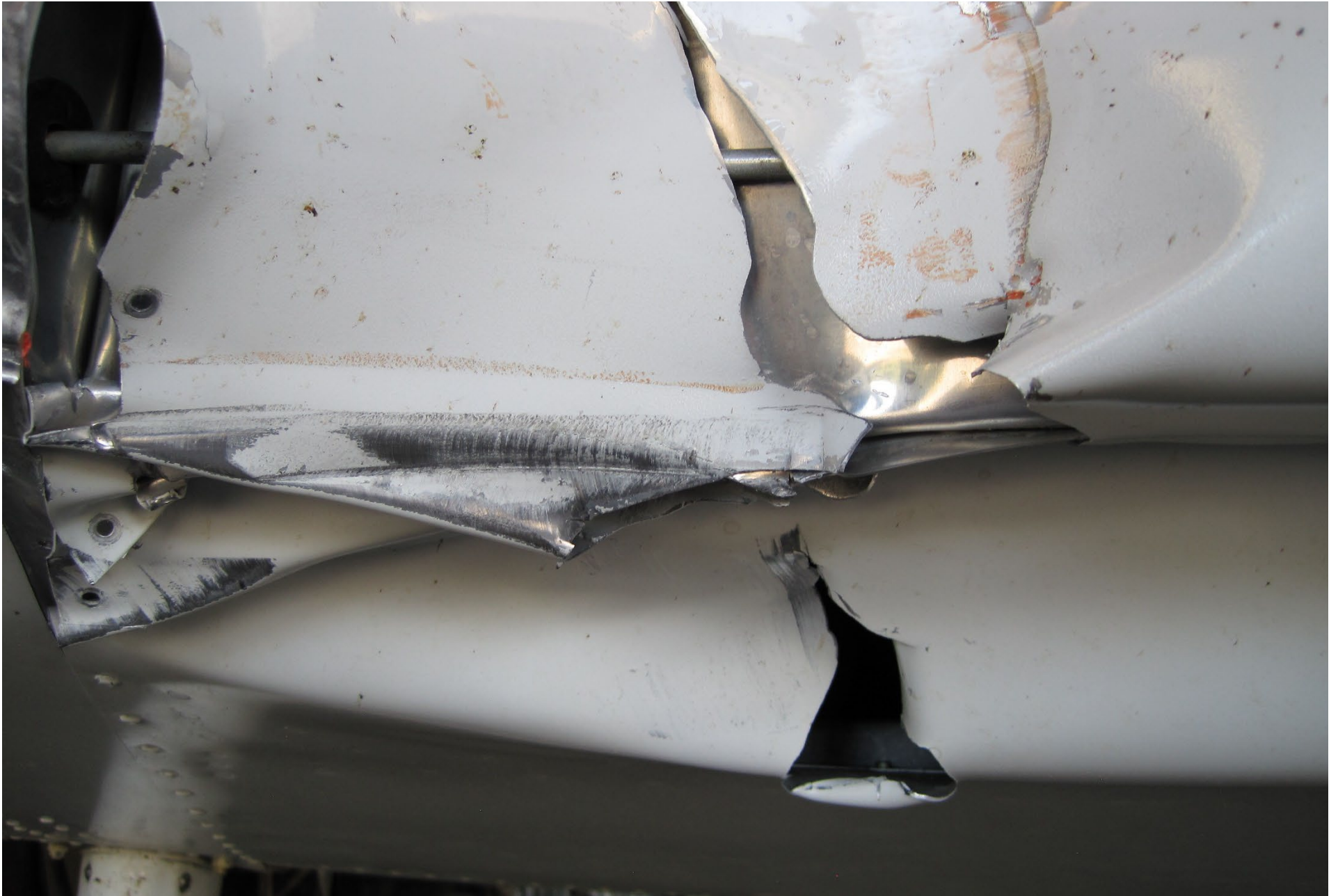
Photo 2 – Bent spar (FAA)
