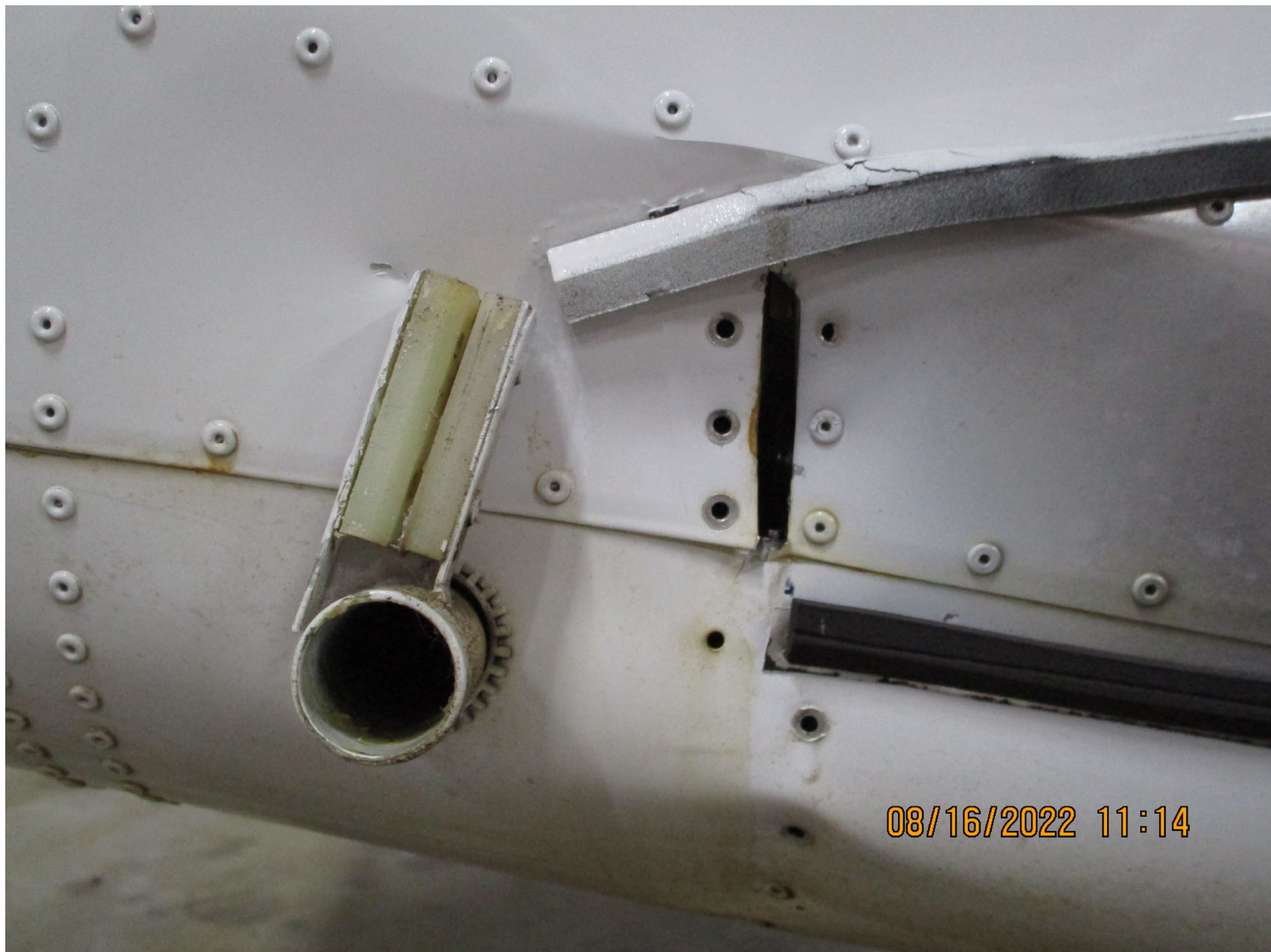
Photo 1 – Damage to the Right Wing (FAA Photo)
