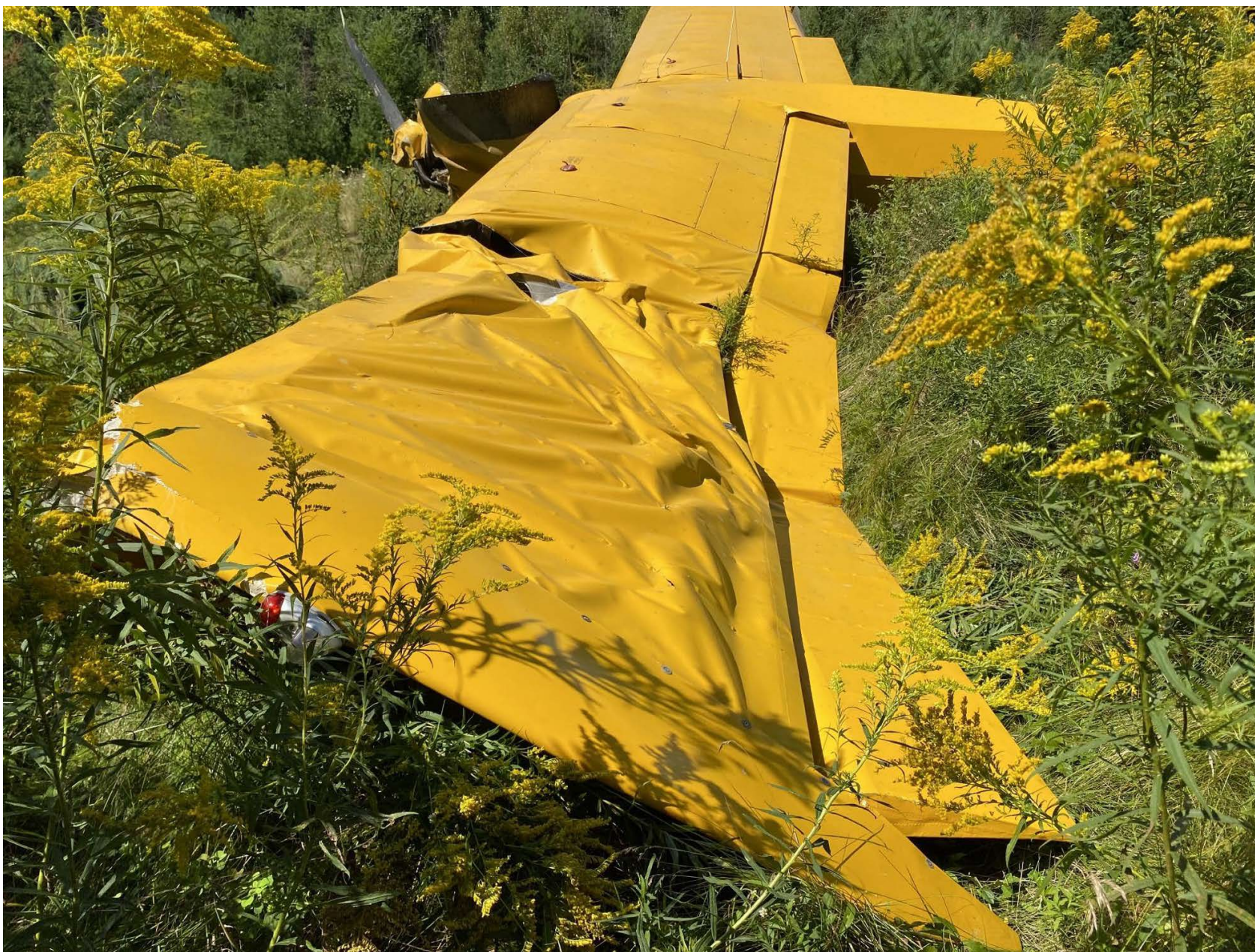
Photo 2 – Top view of damaged left wing (FAA Photo)
