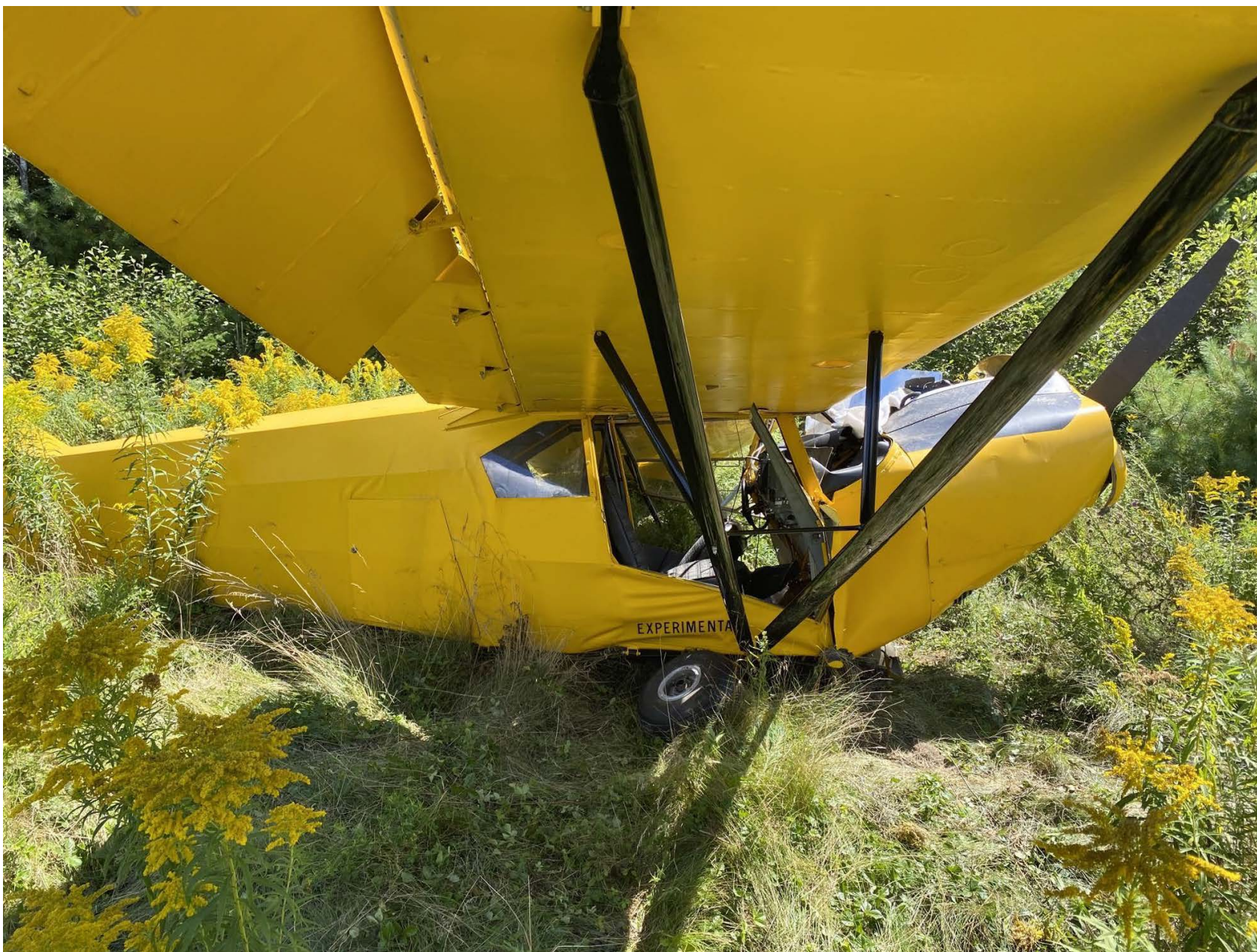
Photo 3 – View right side of damaged fuselage (FAA Photo)
