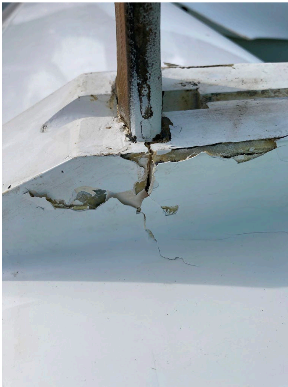
Photo 1 – Torn Tail Section (FAA)
