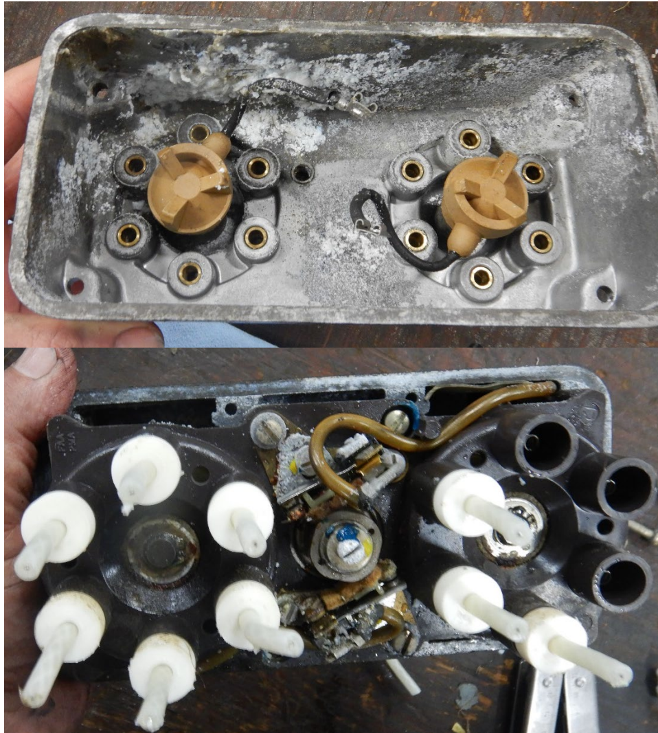
Photograph 6 – Magneto - internal view.
