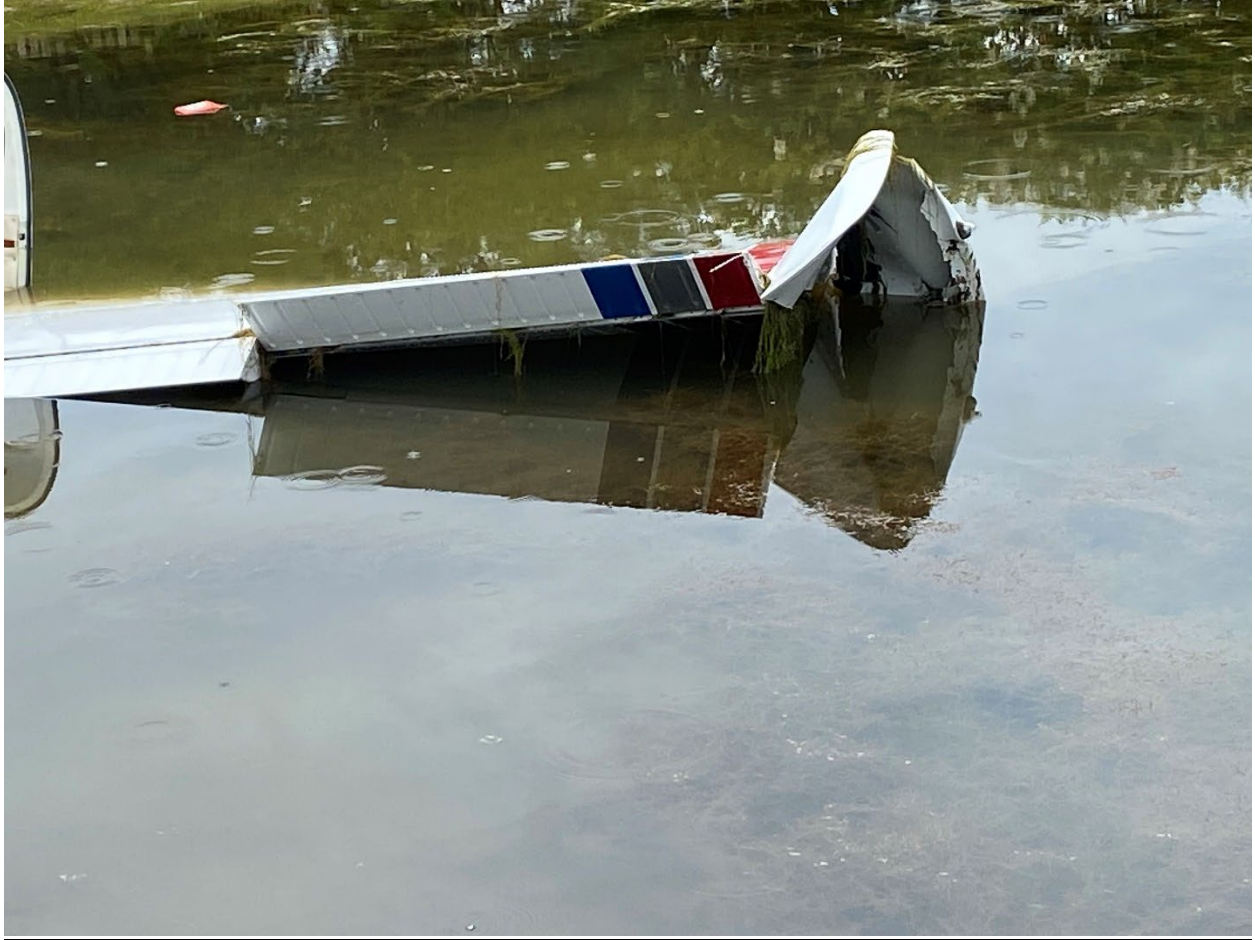
Photograph 3 – Right wing tip damage.
