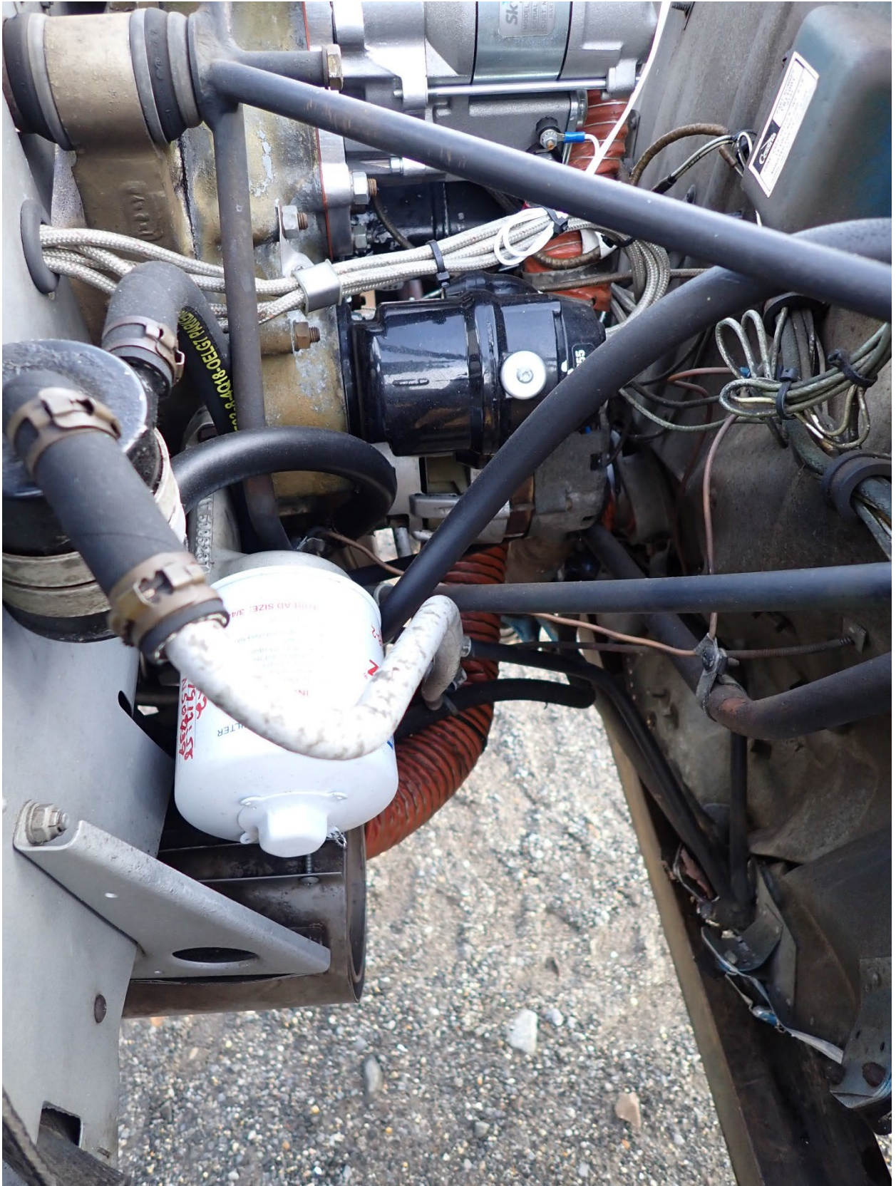
Figure 6: Left magneto attached to accessory case
