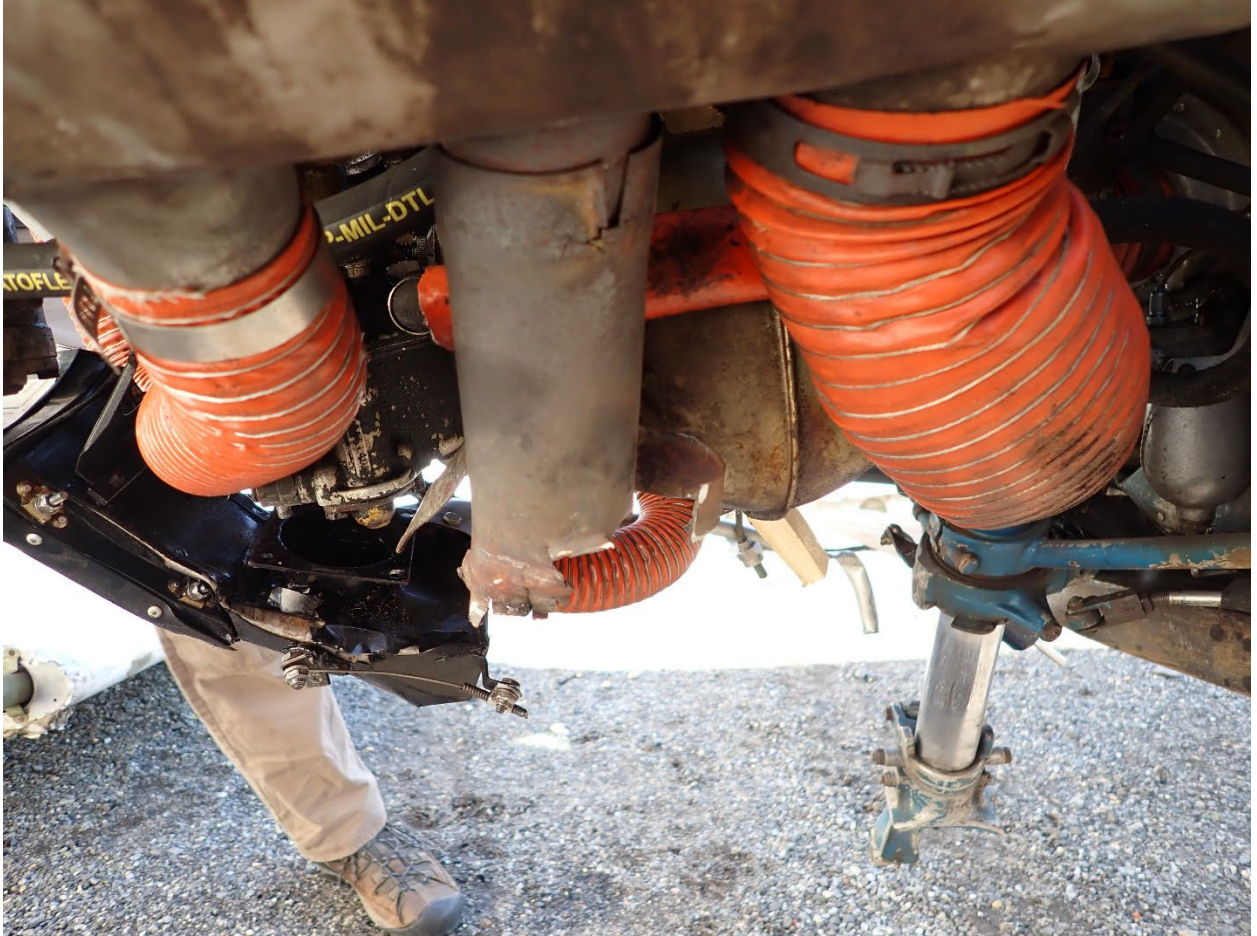
Figure 5: Removed left side exhaust pipe
