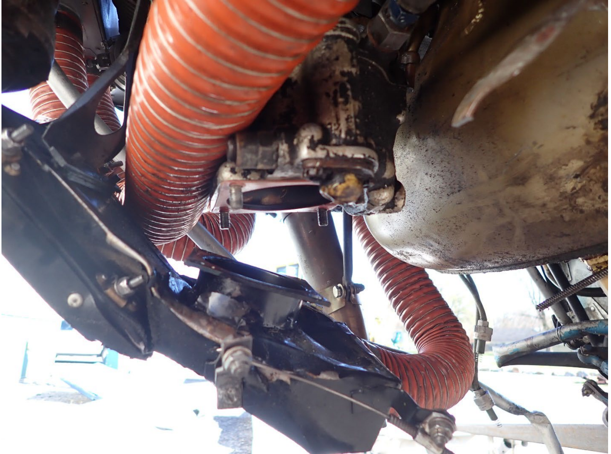
Figure 4: Induction air and carb heat box removed
