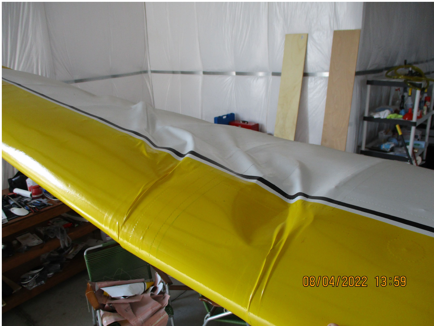
Photo 2 – Wing Damage (FAA Photo)
