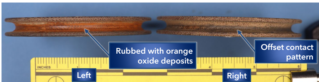
Figure 2. Left and right pulleys from the rudder control system showing the faces with identification markings (upper image) and the cable grooves (lower image).
