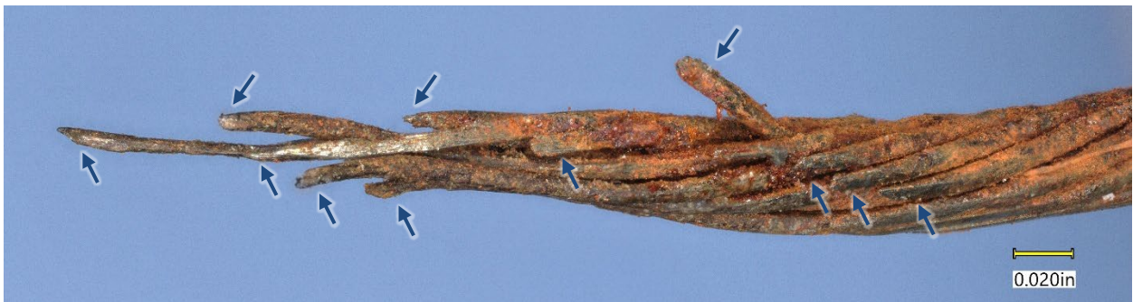
Figure 5. Fractured end of strand 1. Unlabeled arrows indicate worn and fractured wires visible in this view.
