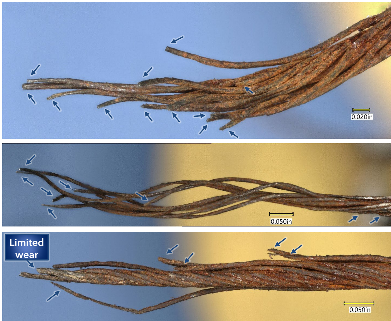
Figure 7. Fractured ends of strands 5 (upper image) and 6 (middle image) and the core strand (lower image). Unlabeled arrows indicate worn and fractured wires visible in these views.
