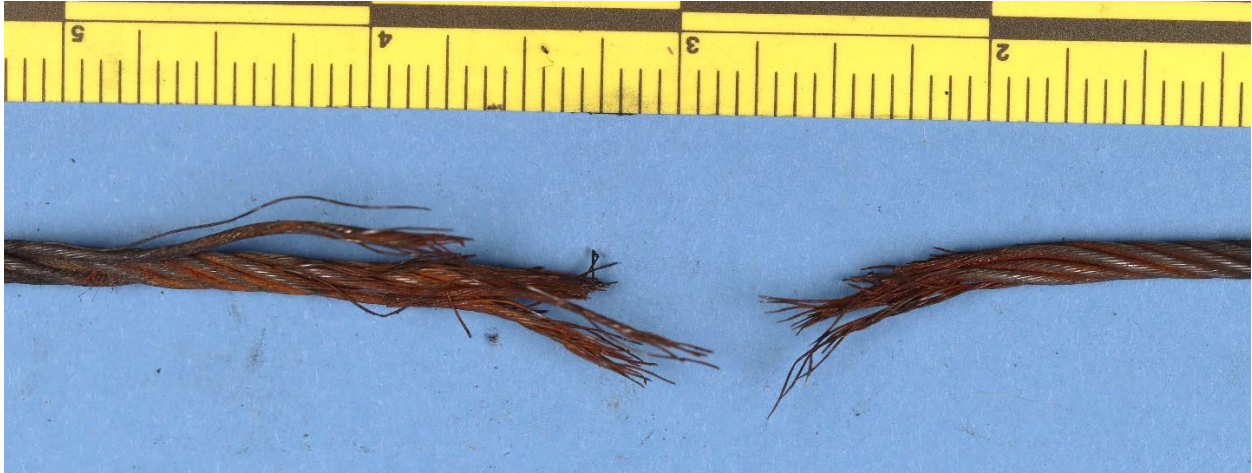
Figure 3. Closer view of the cable fracture indicated in figure 1.
