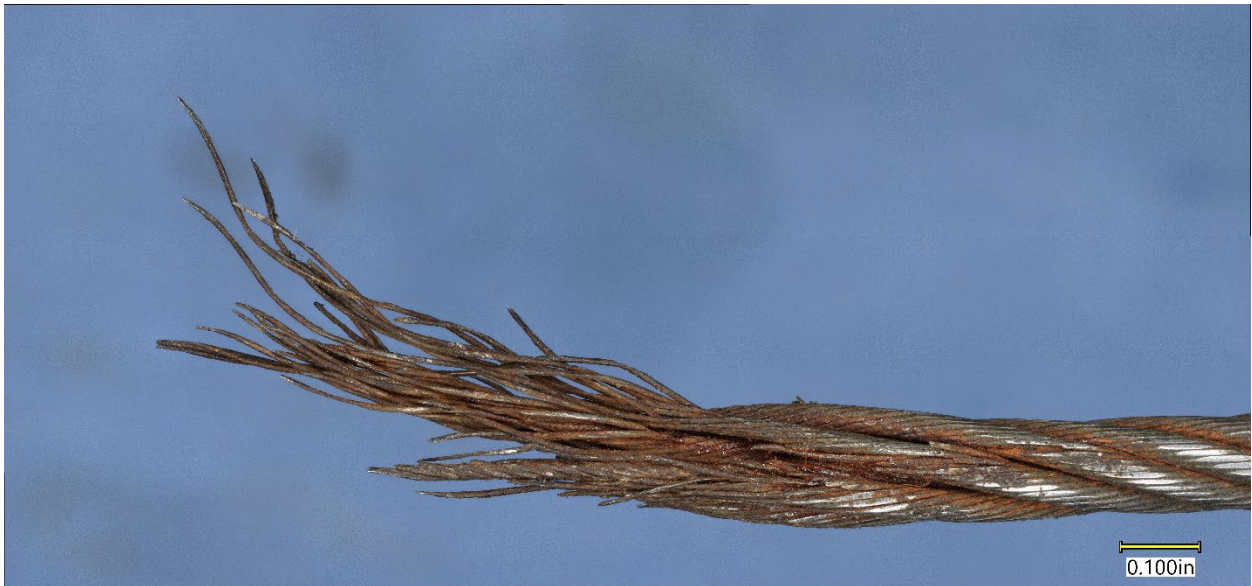
Figure 4. Magnified view of the fracture side shown on the left side of the image in the previous figure.
