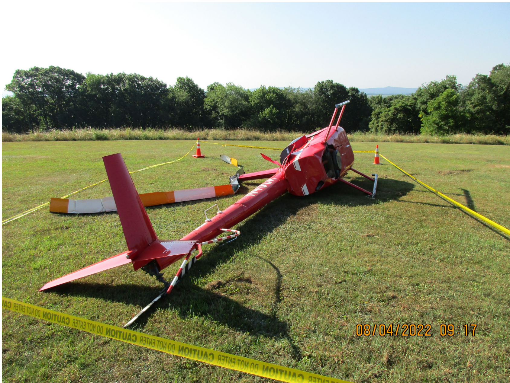
Photo 2 – View of Damage to Tailboom Structure (FAA)
