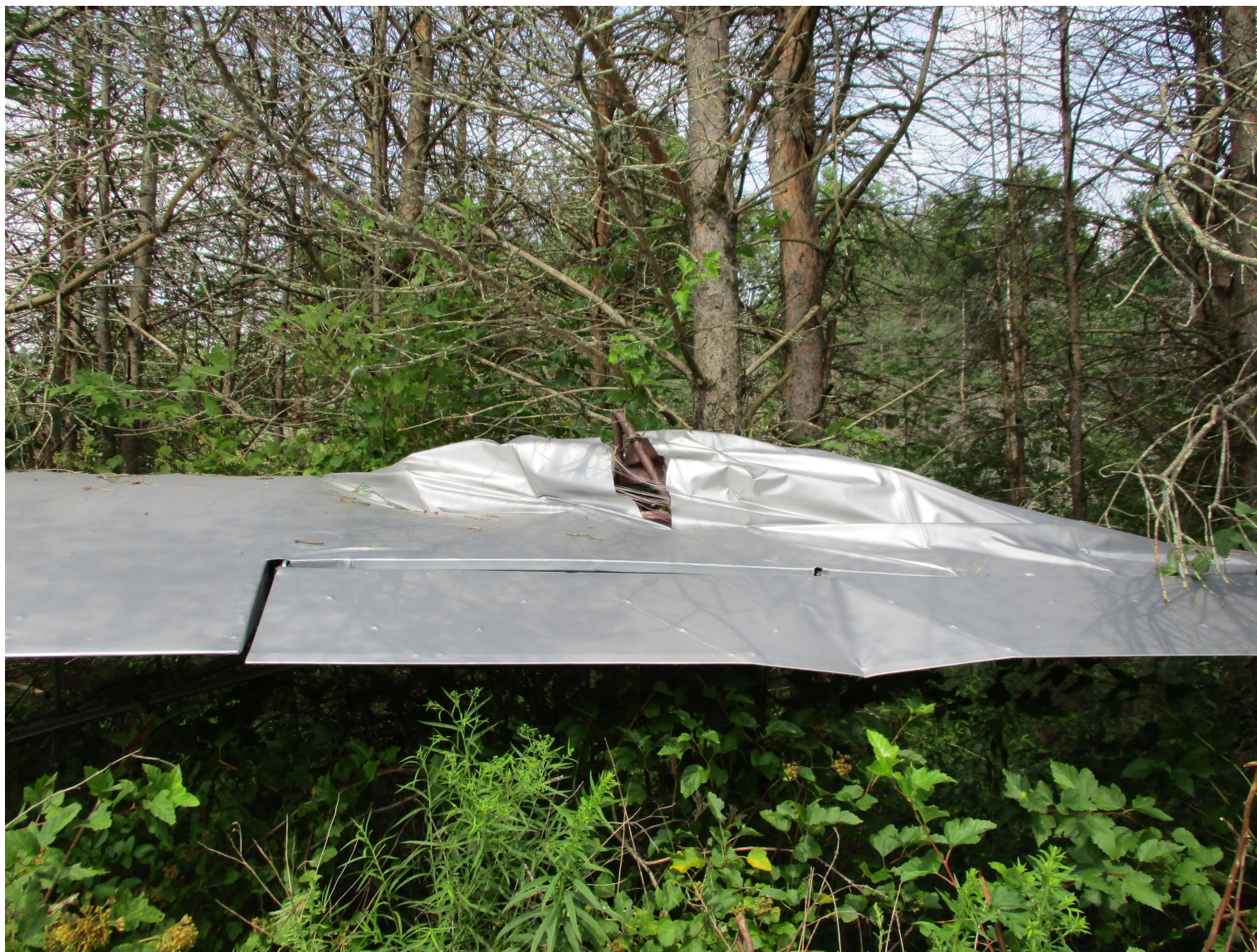
Photo 4: Overview of the damage to the airplane's right wing (Photo Courtesy of FAA)
