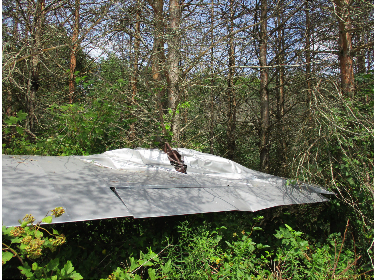
Photo 3: Overview of the damage to the airplane's right wing (Photo Courtesy of FAA)
