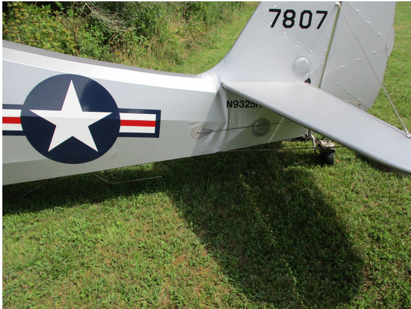
Photo 2: Overview of the damage to the airplane's aft fuselage structure (Photo Courtesy of FAA)
