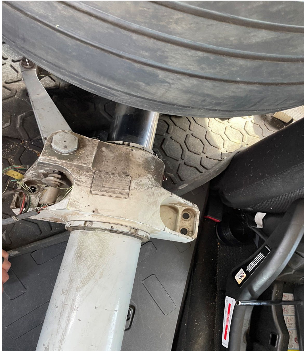
Photo 5 – View of fractured right main landing gear lower attachment points (Photo courtesy of FAA)
