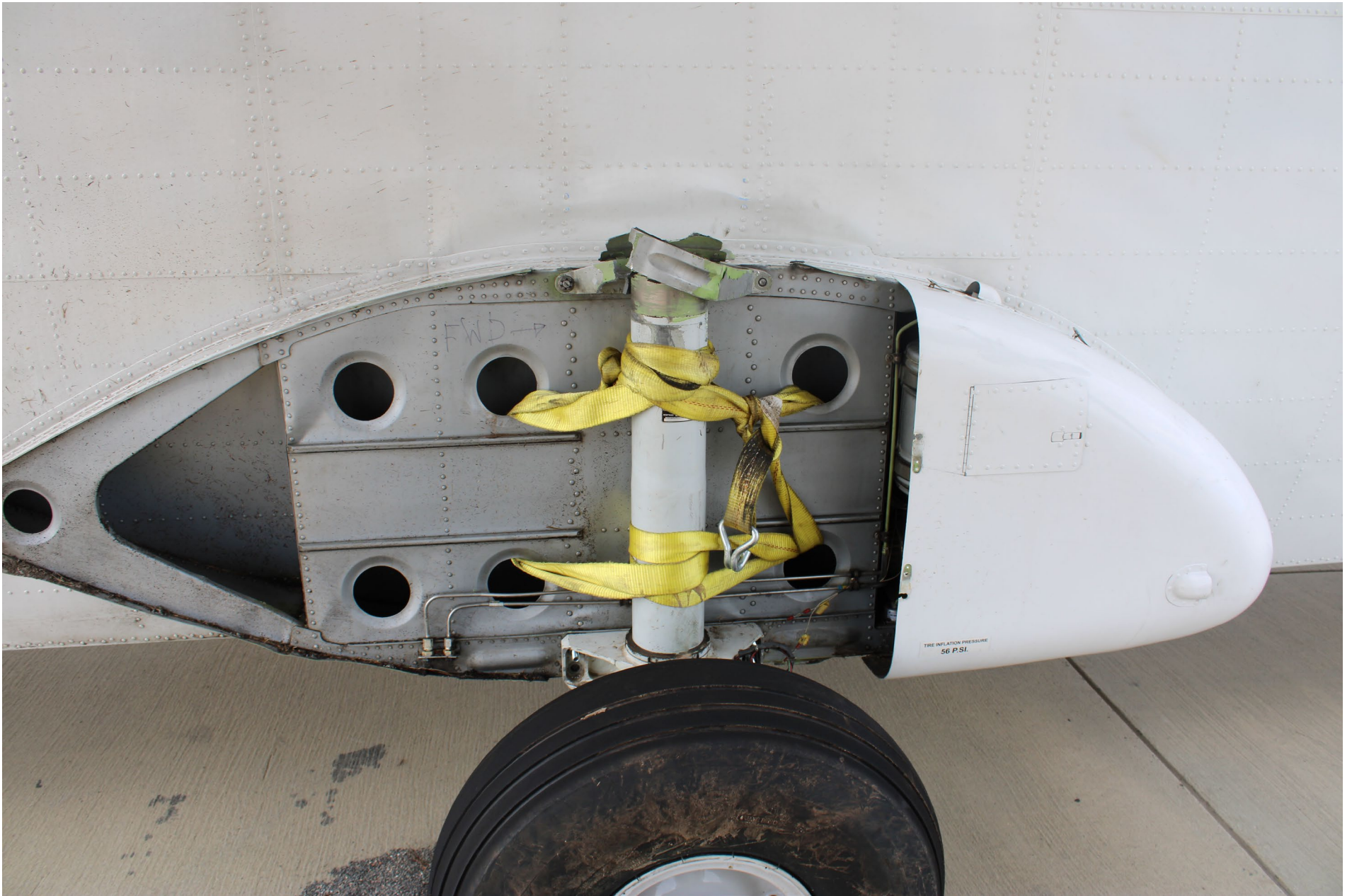
Photo 10 – View of fractured right main landing gear as configured for recovery and ferry
