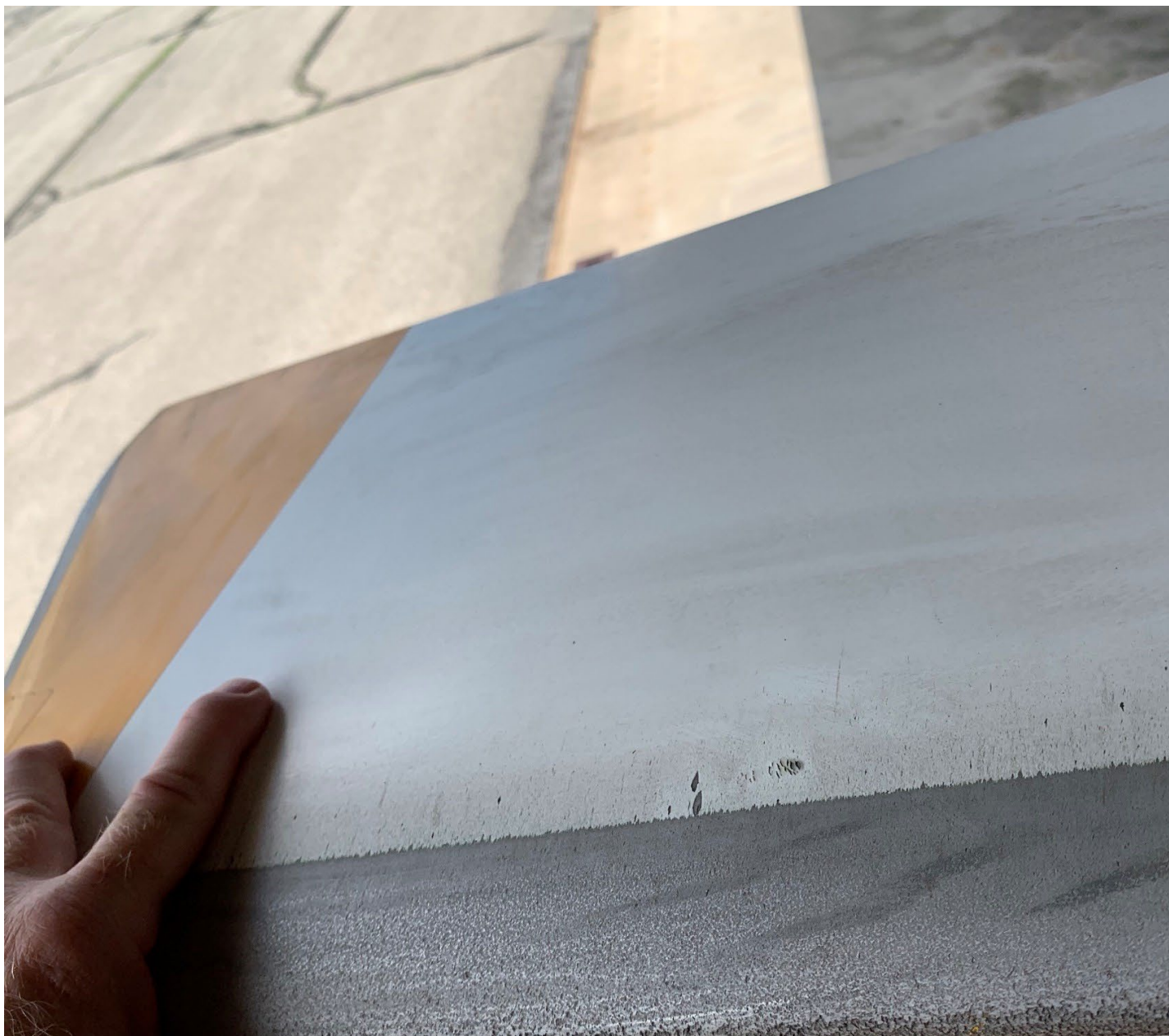
Photo 5 – closeup of main rotor blade (note scoring on blade, courtesy of FAA)
