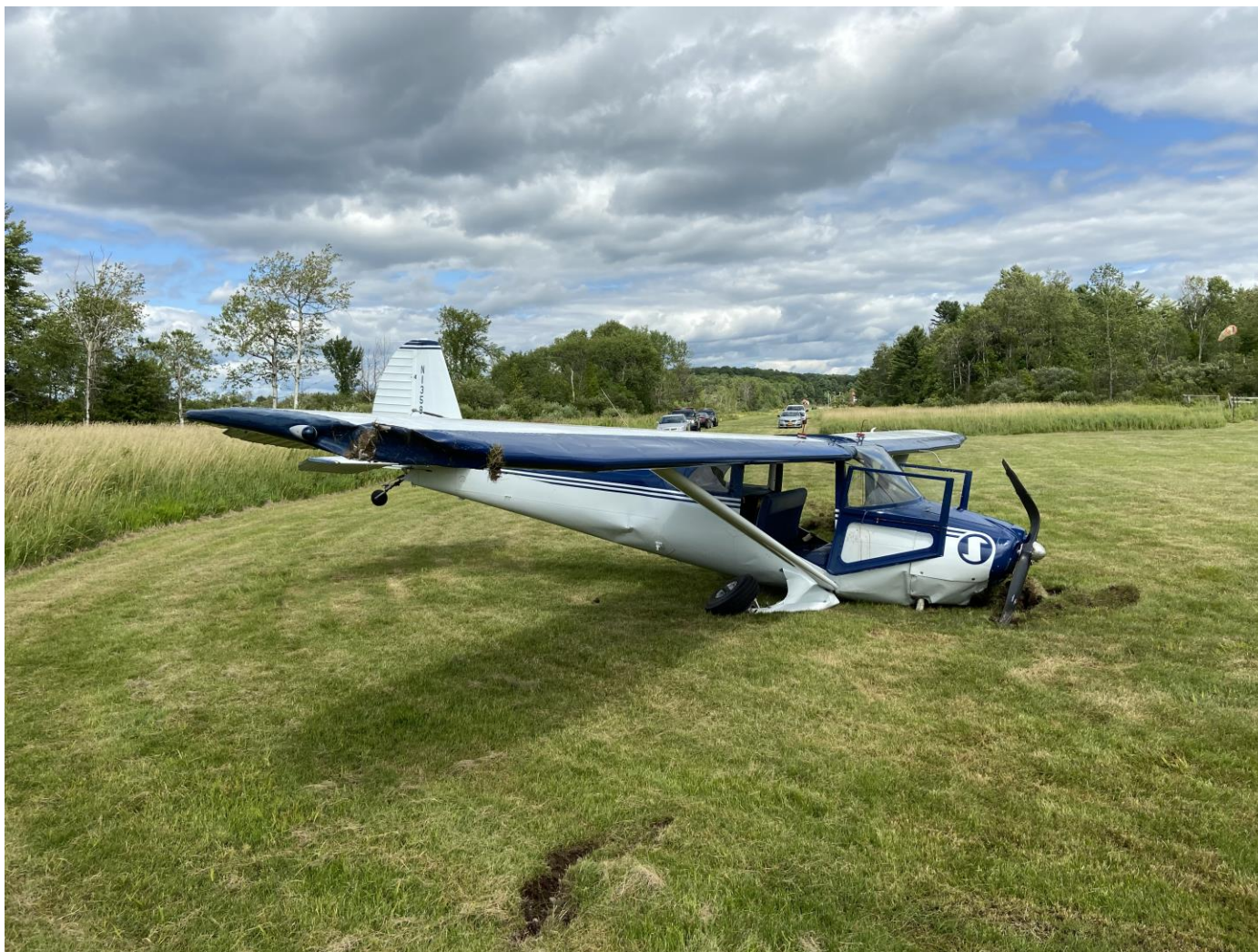
Photograph 3 - Right front quarter view of right wing and airframe damage. (Courtesy of FAA)
