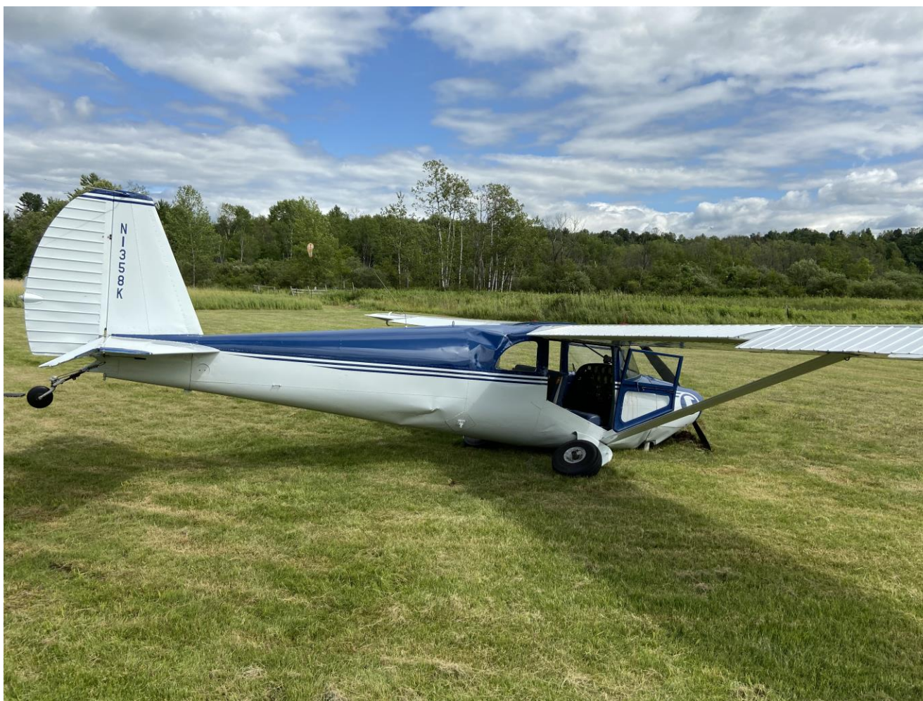
Photograph 2 - Right profile view of airplane damage. (Courtesy of FAA)
