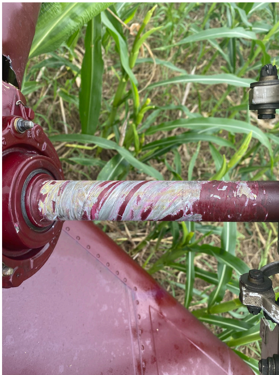
Photo 6 – Cable Wrap Marks on Output Shaft for Tail Rotor – Courtesy of FAA
