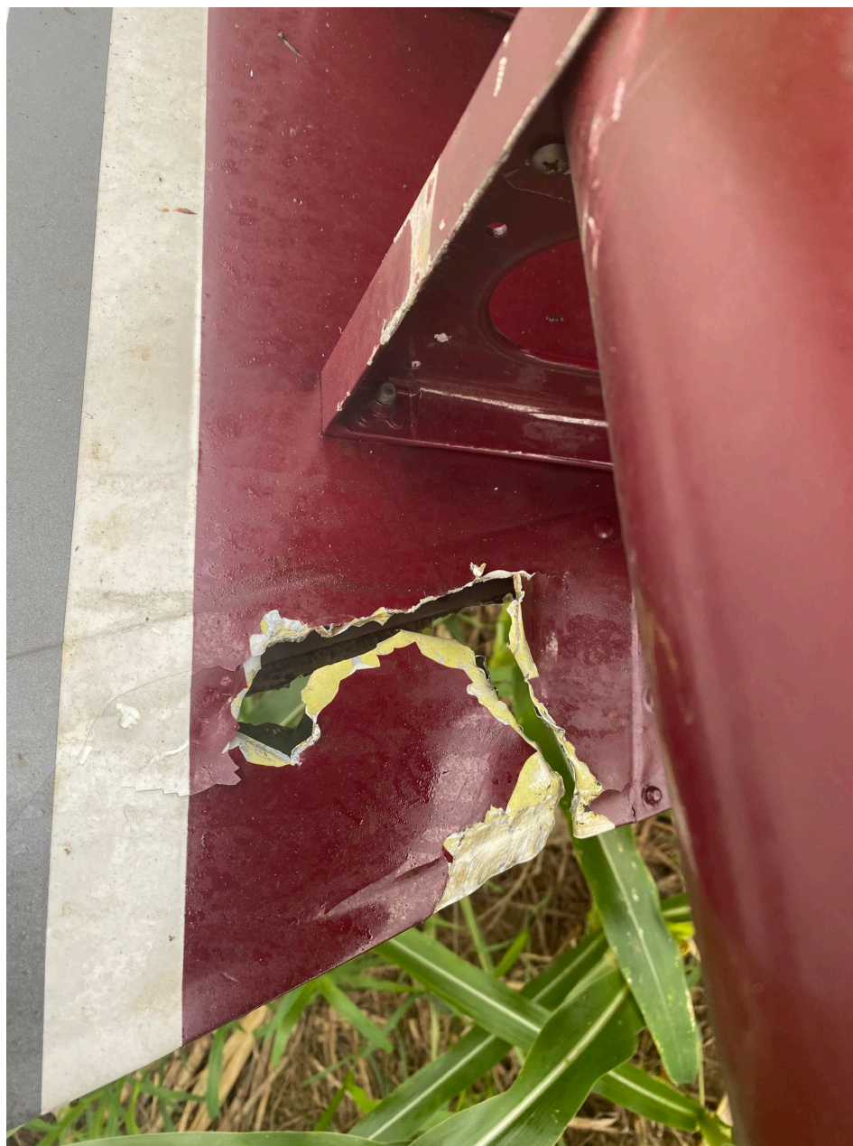
Photo 8 – Cable Penetration on Lower Vertical Stabilizer – Courtesy of FAA
