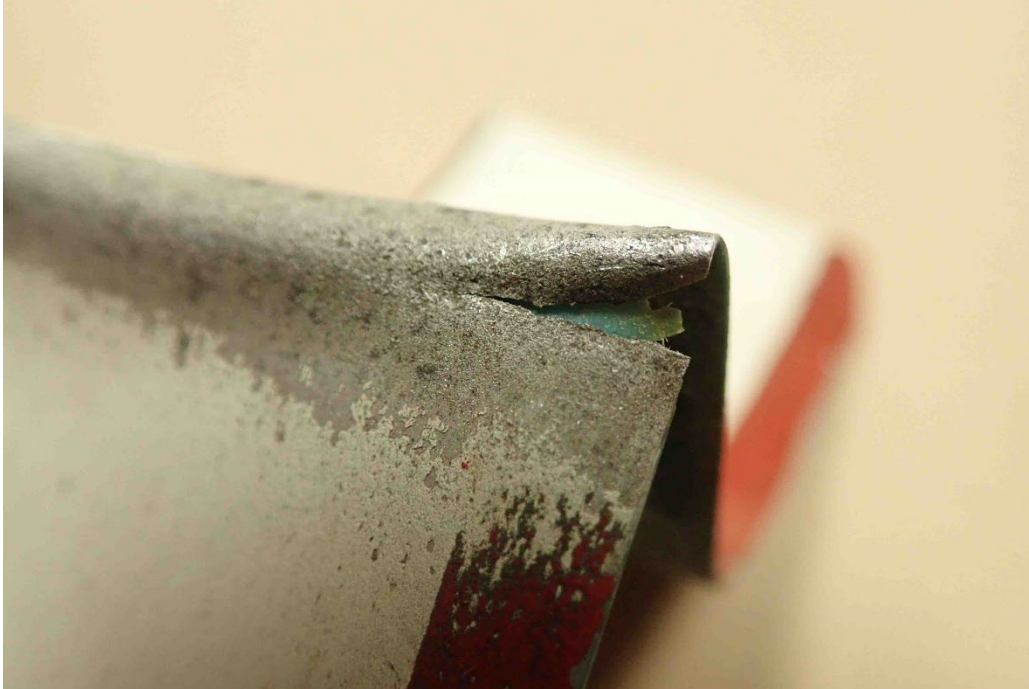
Figure 12 – Leading edge tip crack/tear
