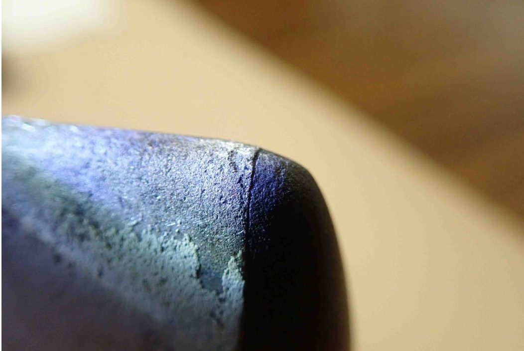
Figure 14 – Tip cap leading edge skin thinning
