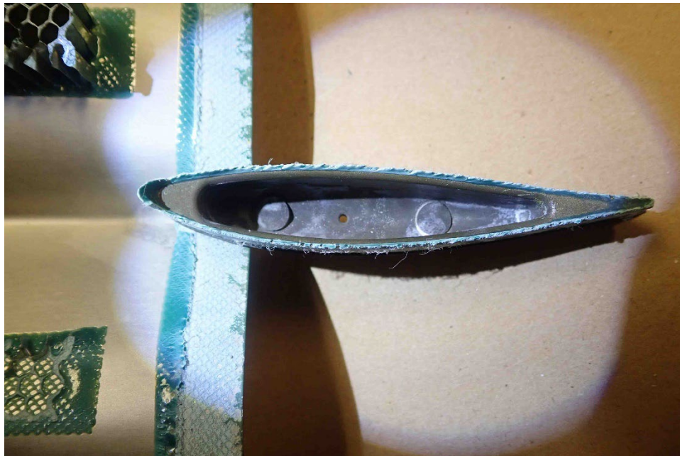
Figure 7 – Tip cap inner surface
