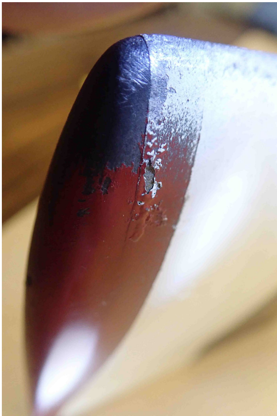
Figure 5 – Corrosion at tip cap
