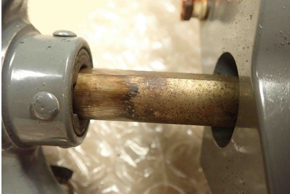
Figure 3- Corrosion to output shaft
