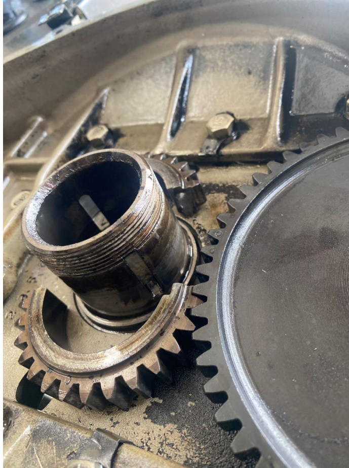
Figure 2: AMF Aviation Digital Photograph. View of the Fractured Crankshaft Gear. Adjacent large gear is Camshaft Gear.
