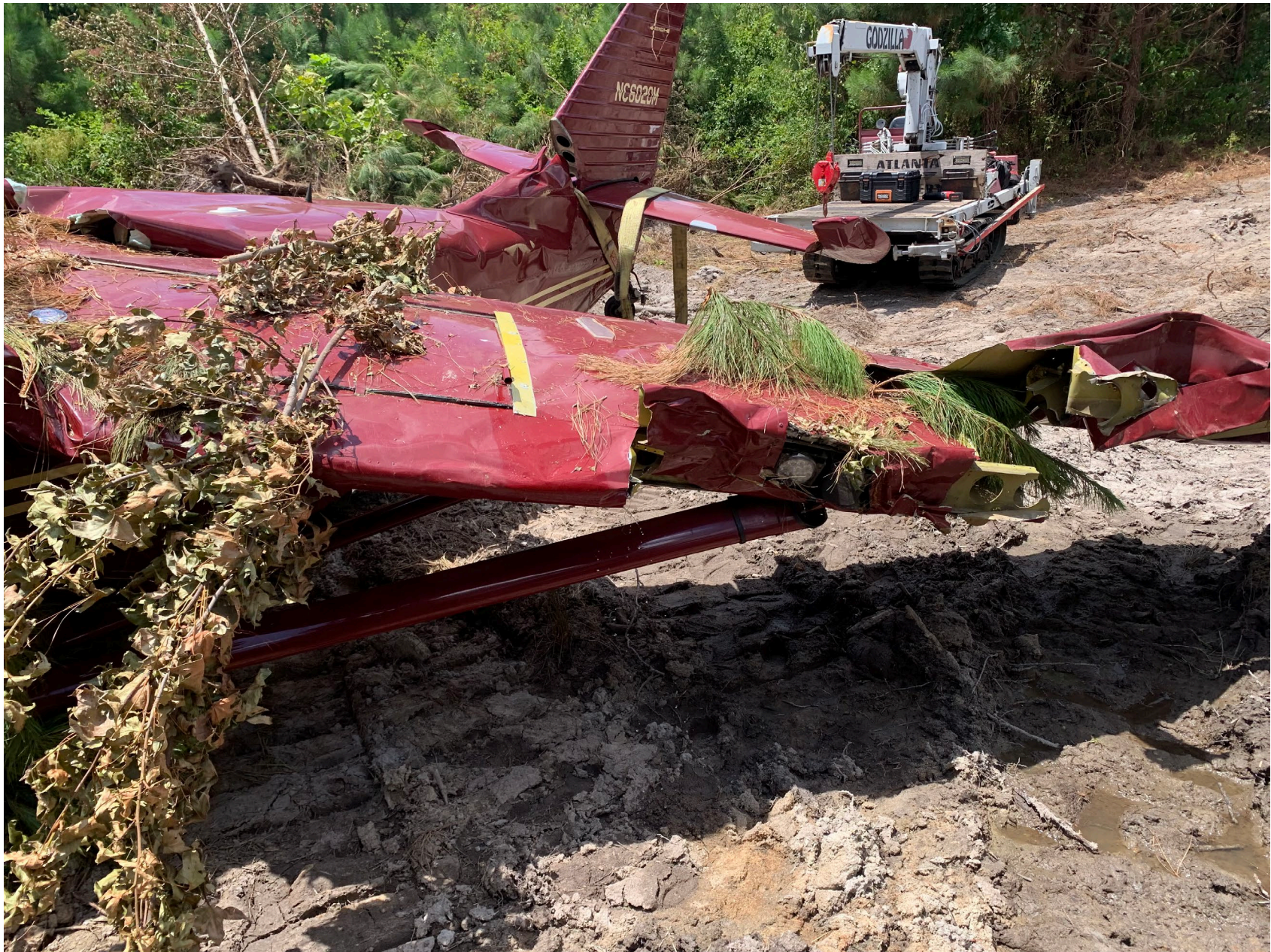
Photo 3 - Digital Photograph From Atlanta Air Salvage. Forward View of Portion of Left Wing Showing Structural Damage to the Main Spar.
