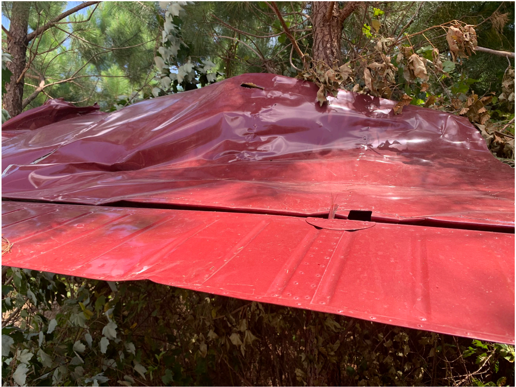
Photo 2 - Digital Photograph From Atlanta Air Salvage. Rear View of Portion of Left Wing Showing Structural Damage.
