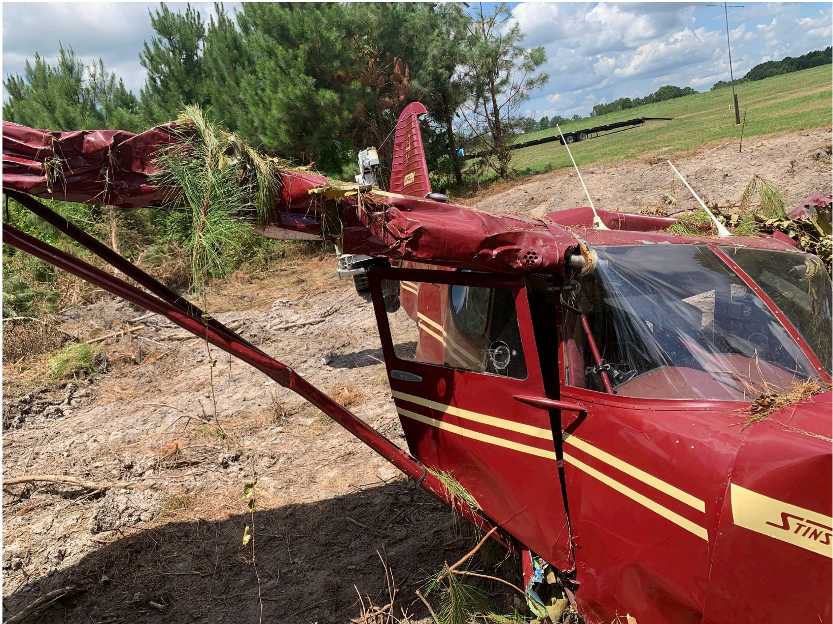
Photo 5 - Digital Photograph From Atlanta Air Salvage. Forward View of the Inboard Portion of the Right Wing Showing Structural Damage to 1 Wing Lift Strut.
