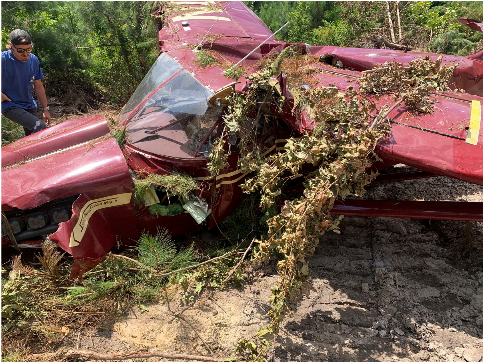
Photo 4 - Digital Photograph From Atlanta Air Salvage. Left Side View Showing Structural Displacement of the Left Wing.
