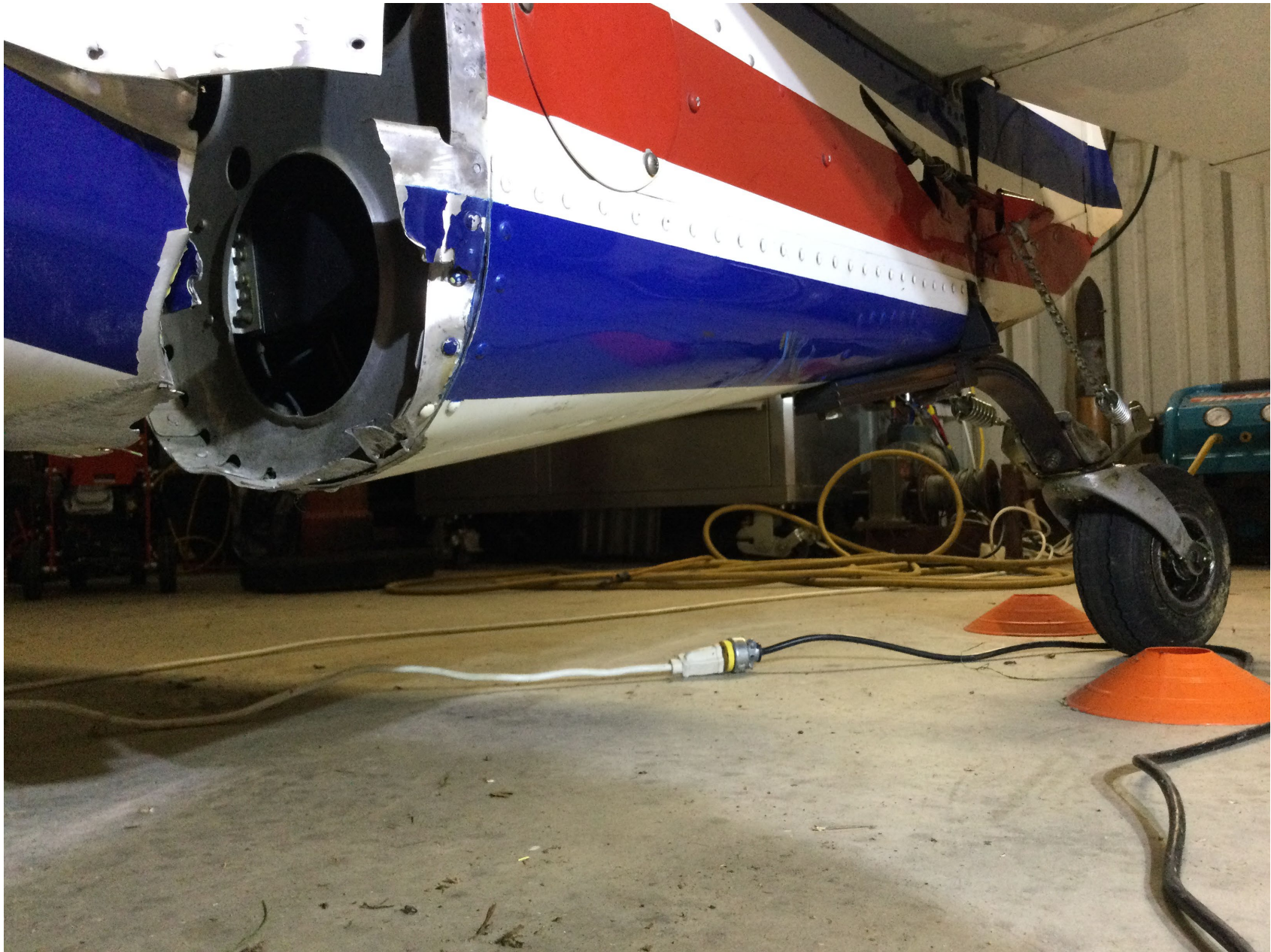
Photo 1 – separation of tail section from fuselage, looking rearward from bottom right (courtesy of FAA)
