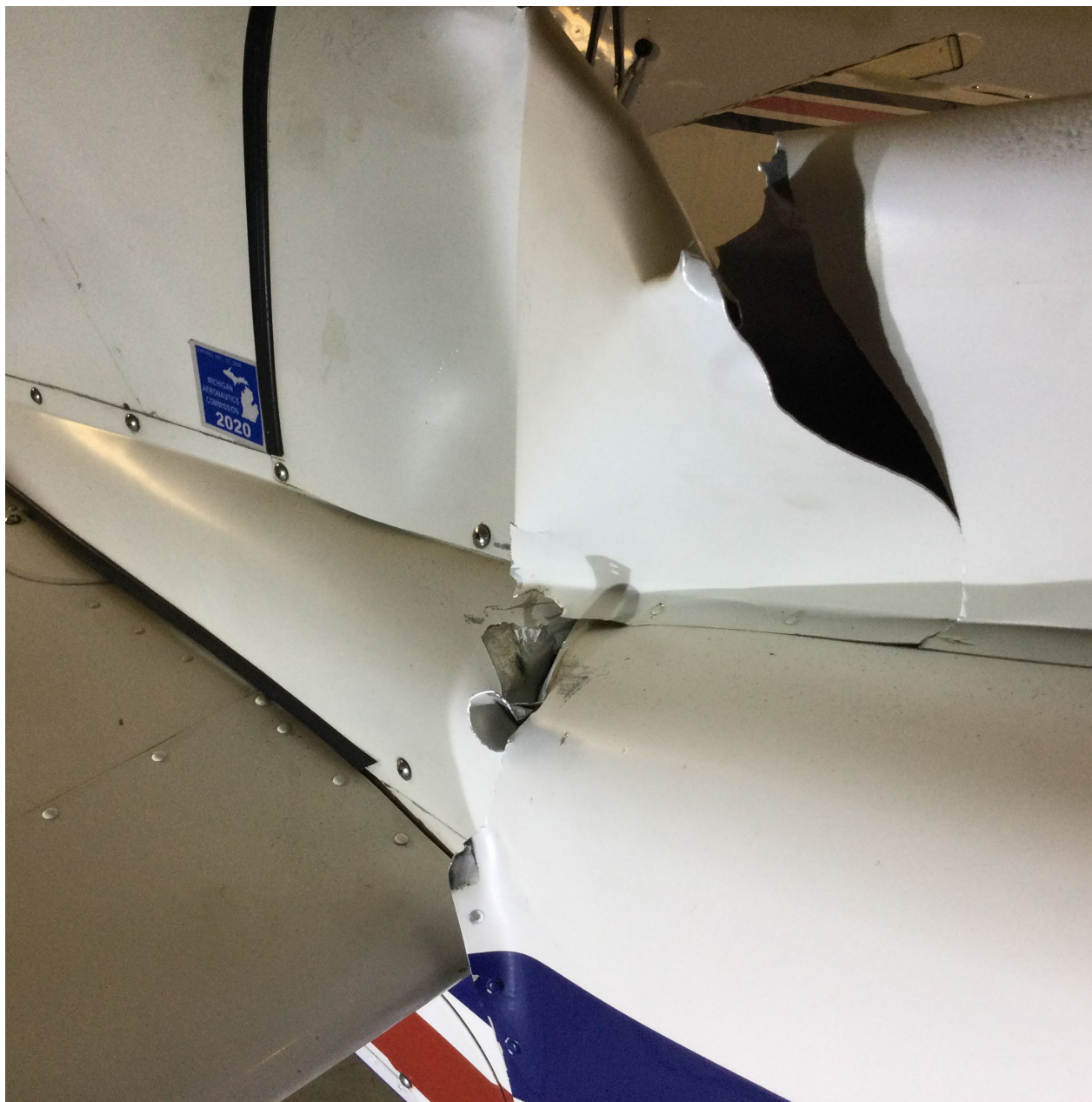
Photo 2 - separation of tail section from fuselage, looking downward from top left (courtesy of FAA)
