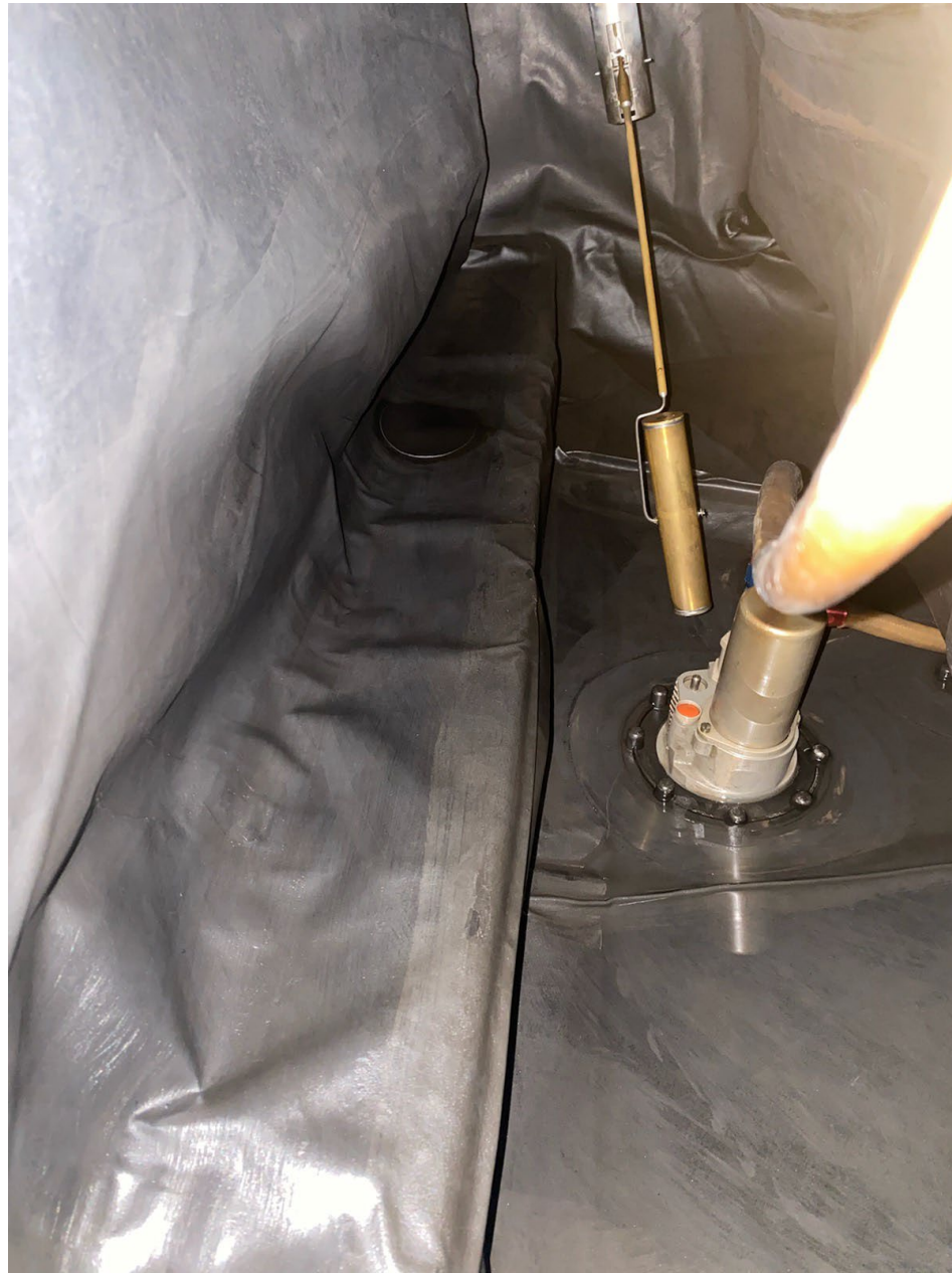
Photo 2 – View of inside fuel cell revealing empty fuel cell (FAA Photo)
