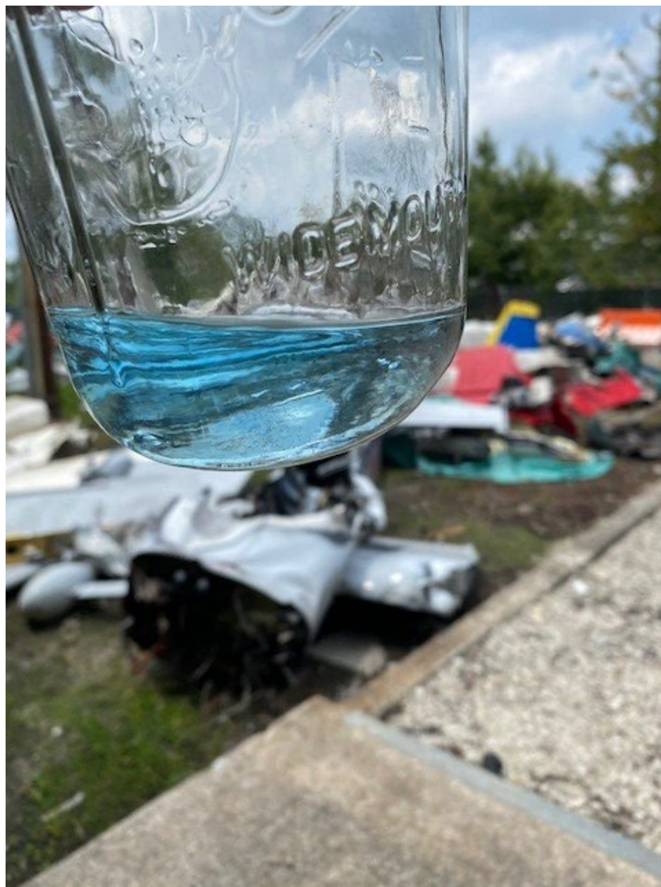
Photo 3 – Fuel Recovered From Gascolator (Photo Courtesy of FAA)
