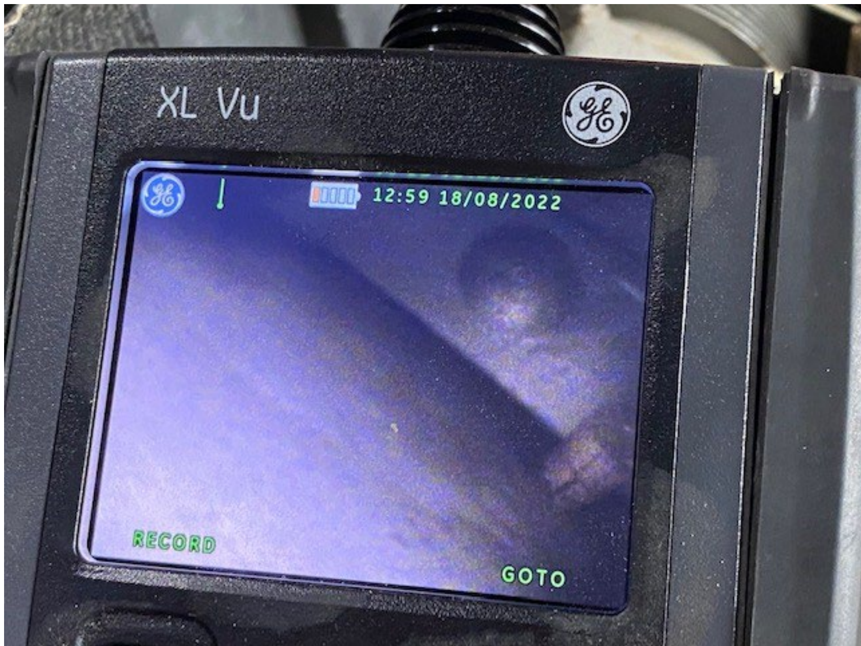
Photo 5 – Empty Section of Fuel Tank (Borecope Photo Courtesy of FAA)
