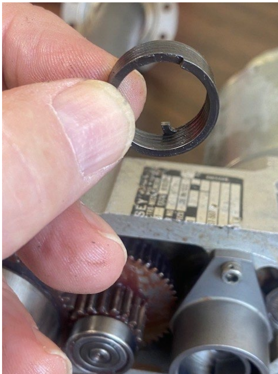
Photo 6 – Digital Photograph From Don Maxwell Aviation. View Depicting Fractured “Tang” of Torsion Spring Inside Clutch Drive Assembly of the Plessey Landing Gear Actuator.
