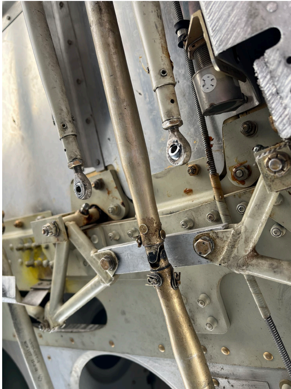
Photo 3 – Digital Photograph From Interstate Turbine. View Depicting the Rods that were Disconnected to Allow the Landing Gear to be Lowered During Recovery of the Airplane From the Runway.
