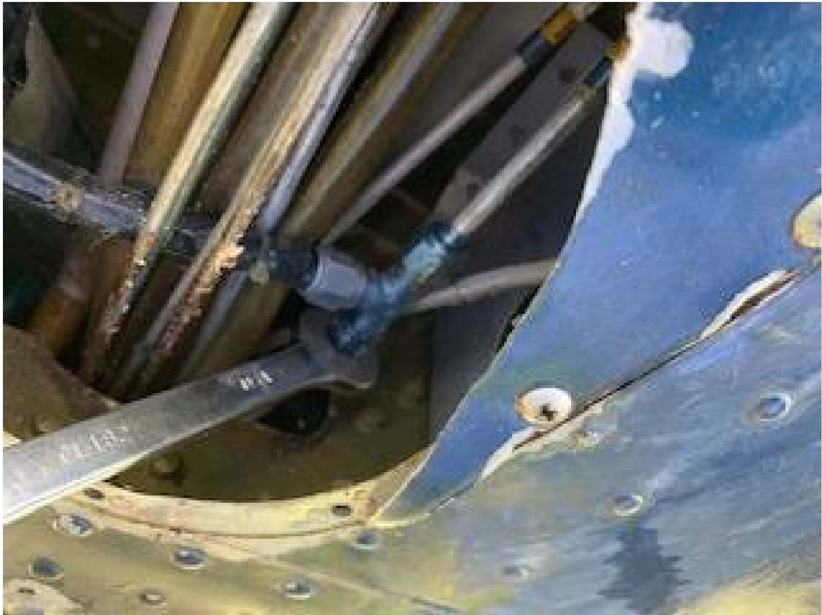
Photo 3 – View of leaking brake line
