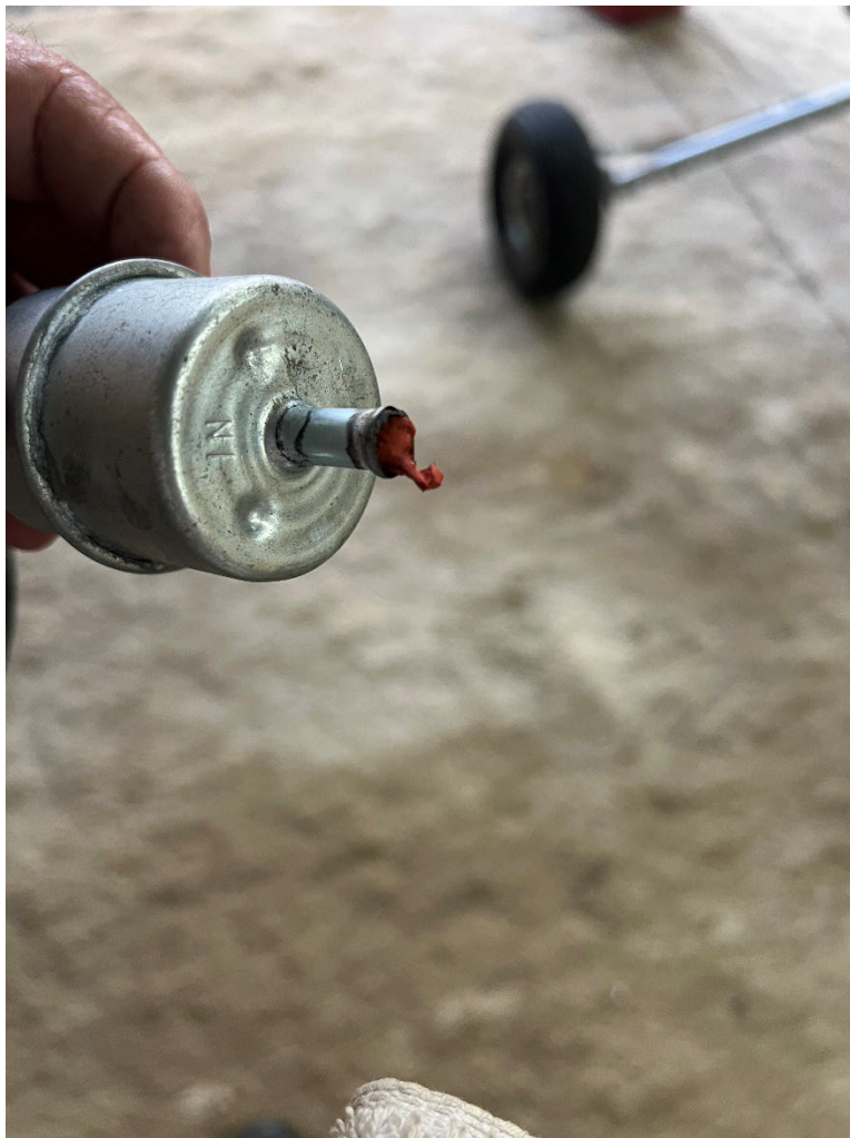
Figure 1: Digital Photograph From Pilot. View Depicting Foreign Object in Fuel Filter Inlet Fitting.
