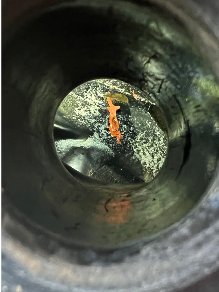
Figure 4: Digital Photograph From Pilot. View Looking Inside The Fuel Tank. Note the Same Colored Material in the Bottom Of the Fuel Tank as Was Found in the Fuel Filter Inlet.
