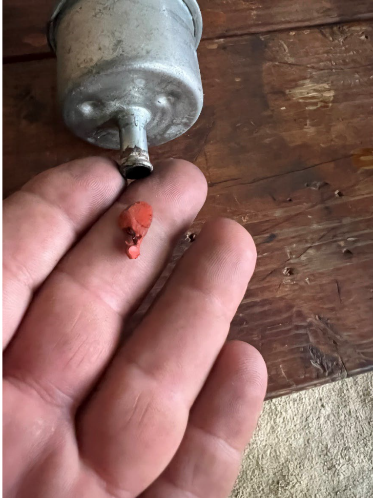
Figure 2: Digital Photograph From Pilot. View Depicting Foreign Object Removed From Fuel Filter Inlet.
