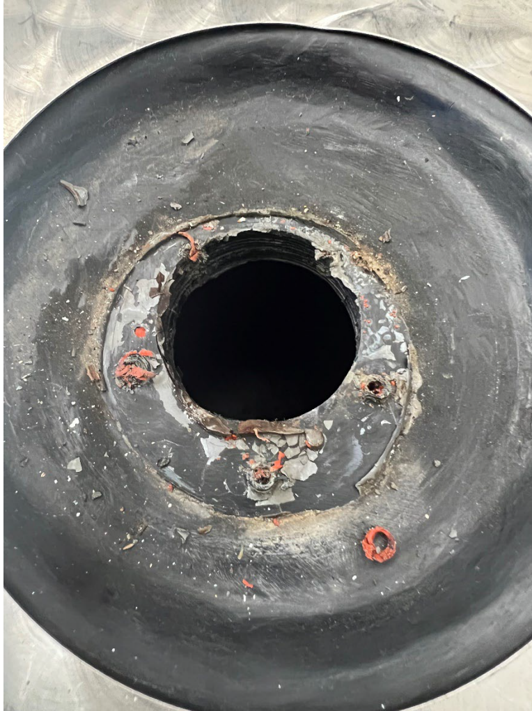
Figure 3: Digital Photograph From Pilot. View Depicting The Fuel Tank Opening Where Fuel Sending Unit is Installed. Note The Similar Colored Sealant Found in the Fuel Filter Inlet.
