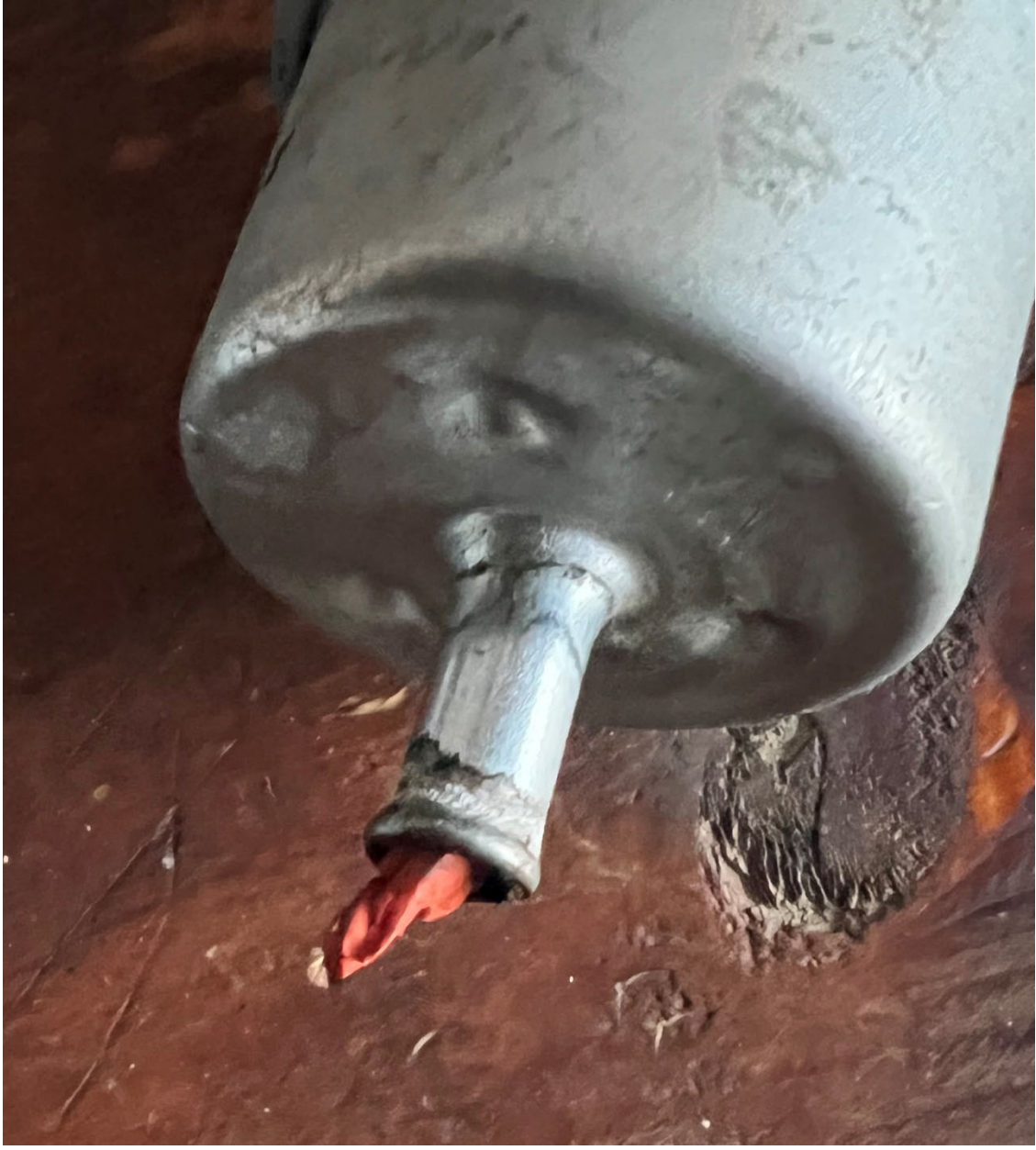
Photograph 2 – Foreign material found in fuel filter.
