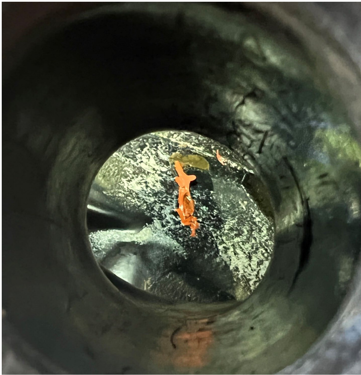
Photograph 4 – Foreign material found in fuel tank.
