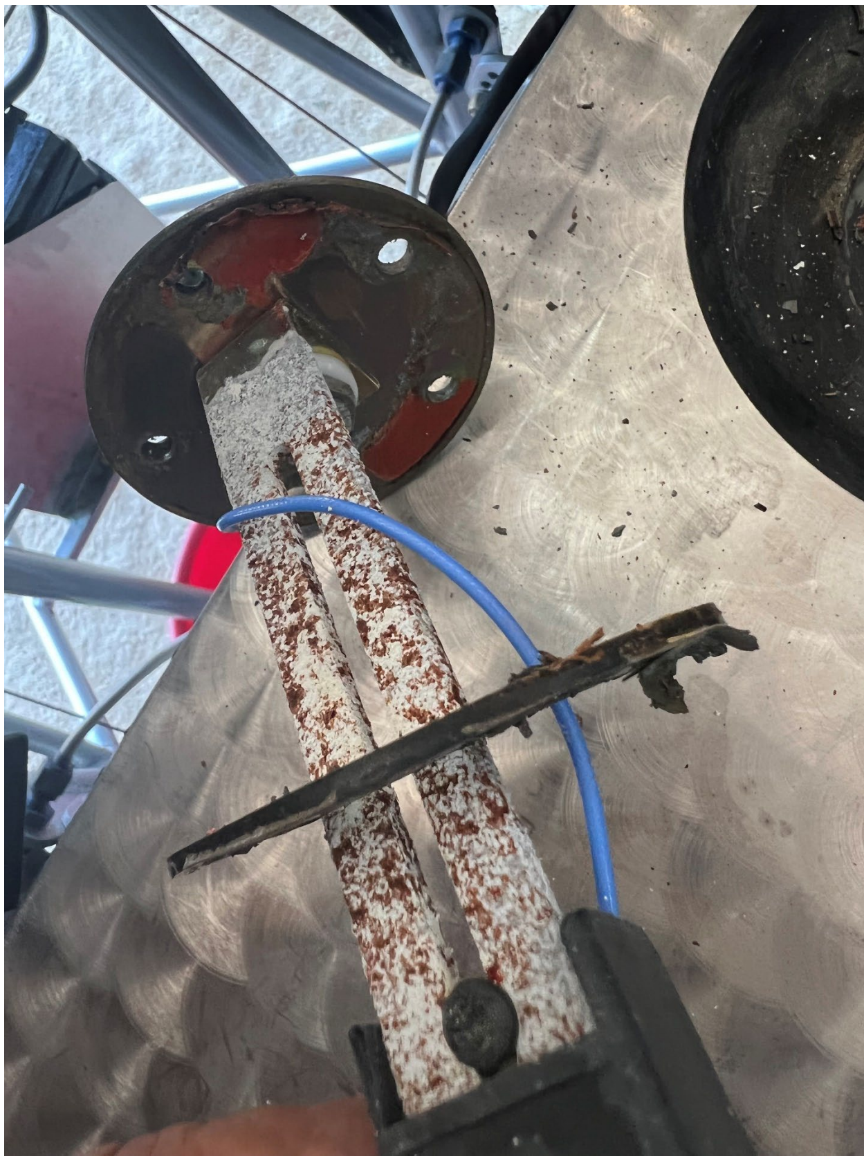
Photograph 3 – Fuel sending unit.
