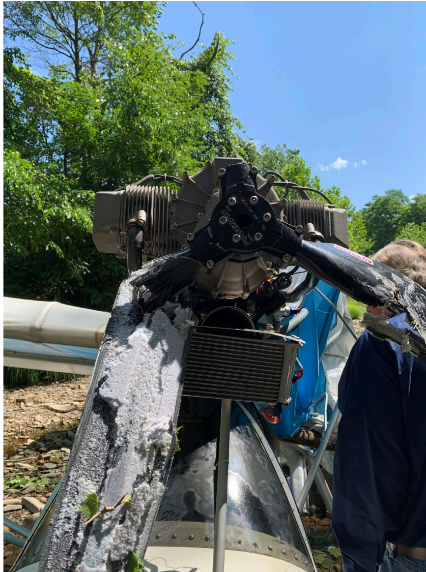
Photograph 3 - View of damaged and shattered propeller blades. (Courtesy of FAA)
