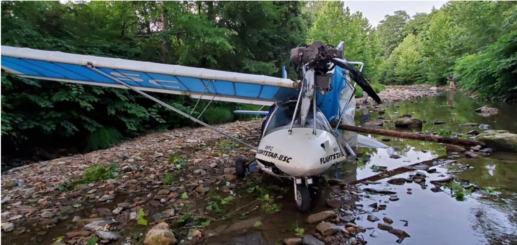
Photograph 2 - Front view of airplane damage and fractured left wing. (Courtesy of FAA)
