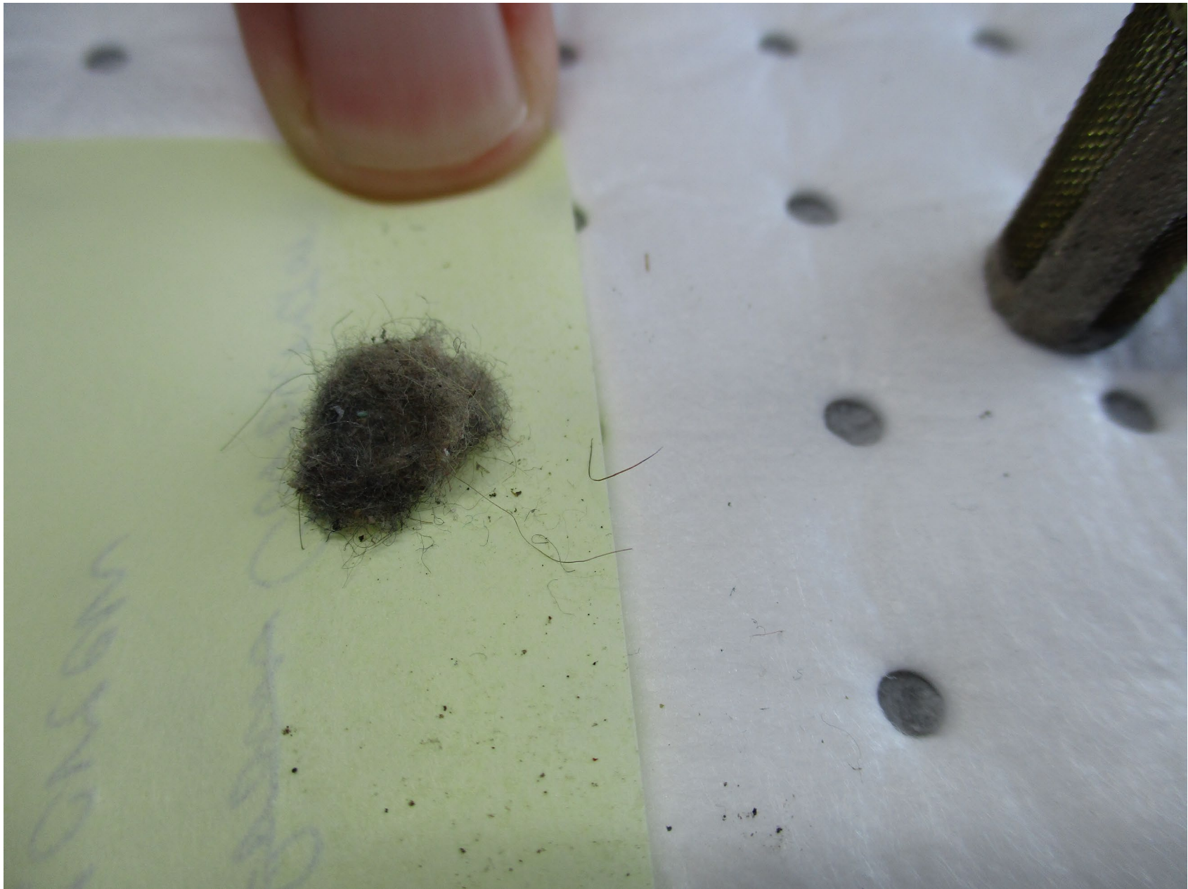
Photo 11 - FAA Digital Photograph. View of the Material removed From the Carburetor Inlet Screen.
