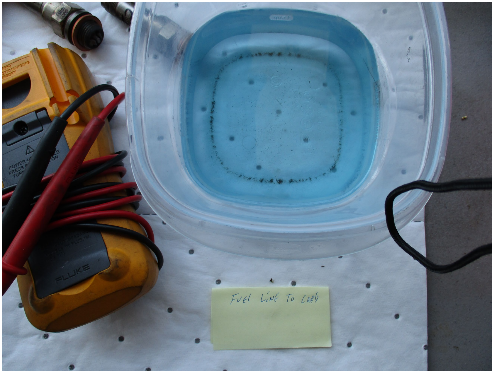
Photo 14 - Annotated FAA Digital Photograph. View of the Fuel Drained From the Fuel Line to the Carburetor. Note the Contaminants (Black Particulates).
