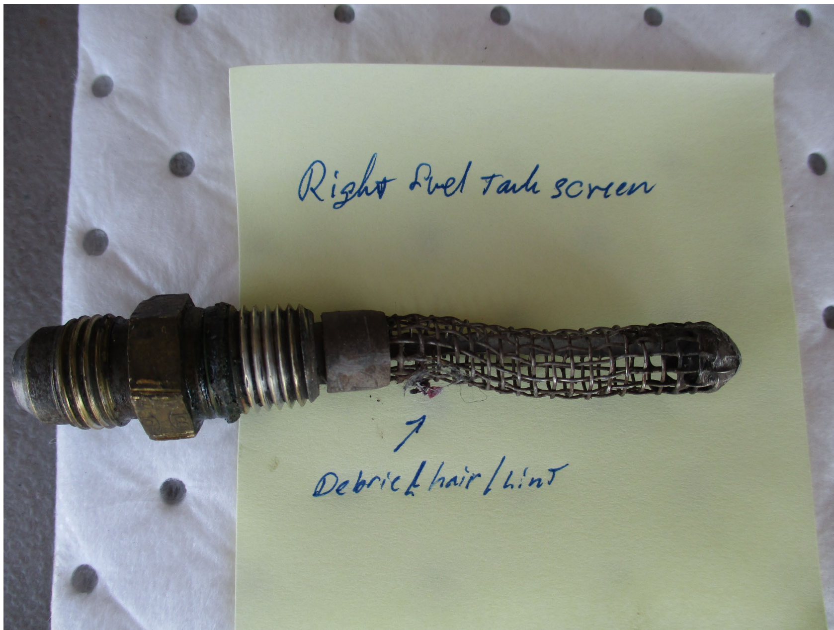
Photo 13 - Annotated FAA Digital Photograph. View of the Right Fuel Tank Strainer. Note the debris Near the End of the Screen Close to the Outlet Fitting.
