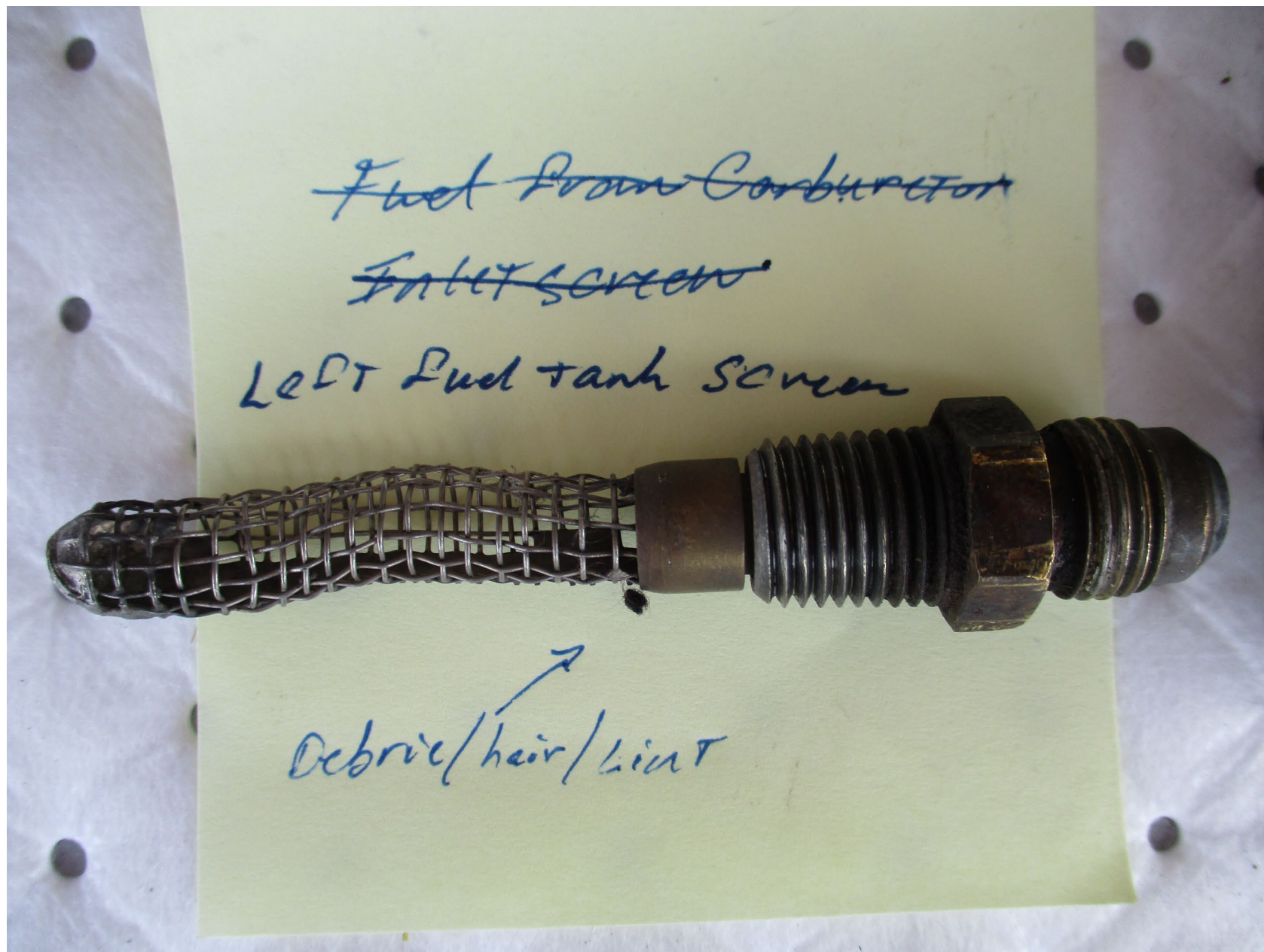
Photo 12 – Annotated FAA Digital Photograph. View of the Left Fuel Tank Strainer. Note the debris Near the End of the Screen Close to the Outlet Fitting.
