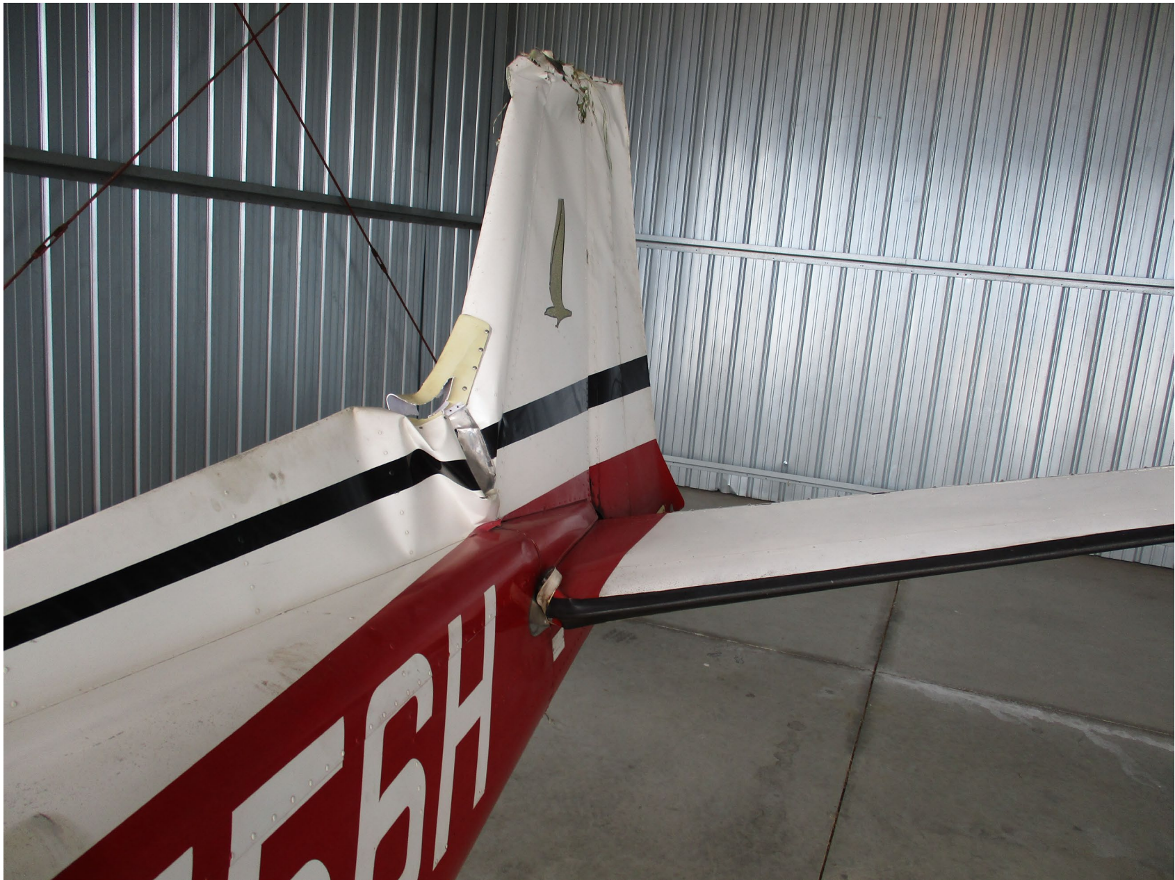
Photo 5 - FAA Digital Photograph. Left Side View Depicting the Aft Empennage, Portion of Left Horizontal Stabilizer, Vertical Stabilizer and Rudder. Note the Damage to the top Part of the Vertical Stabilizer.
