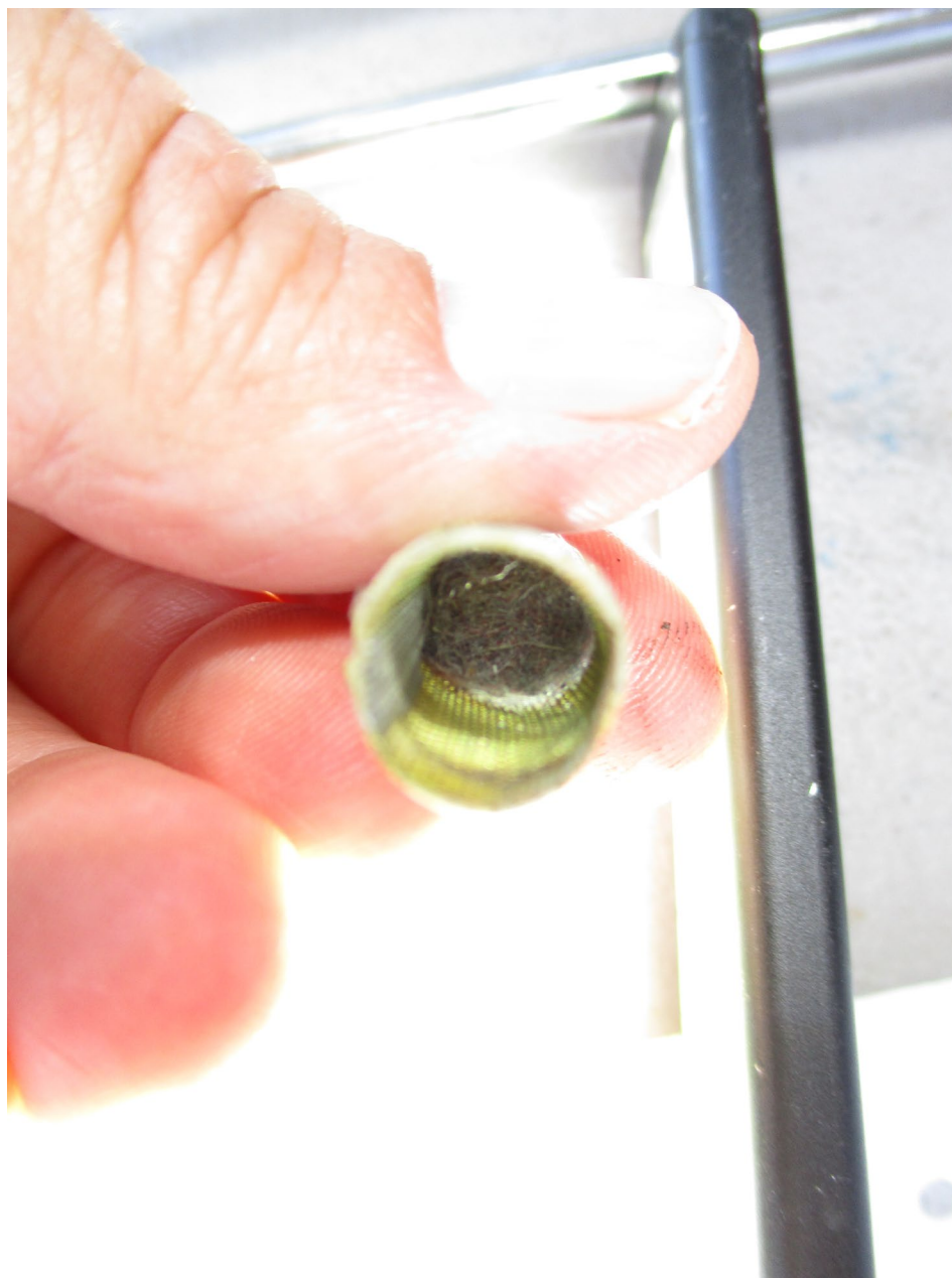
Photo 10 - FAA Digital Photograph. View of the Carburetor Inlet Screen. Note the Material Inside the Screen at the End.
