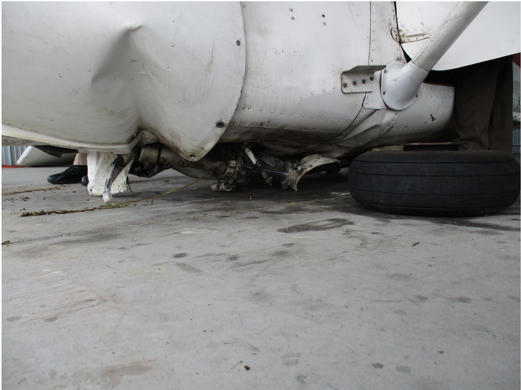
Photo 2 - FAA Digital Photograph. Left Forward Quartering View of the Lower Left Front part of the Fuselage. Note the Compression Buckling in the Structure Adjacent to the Left Wing Lift Strut Lower Attach Point.
