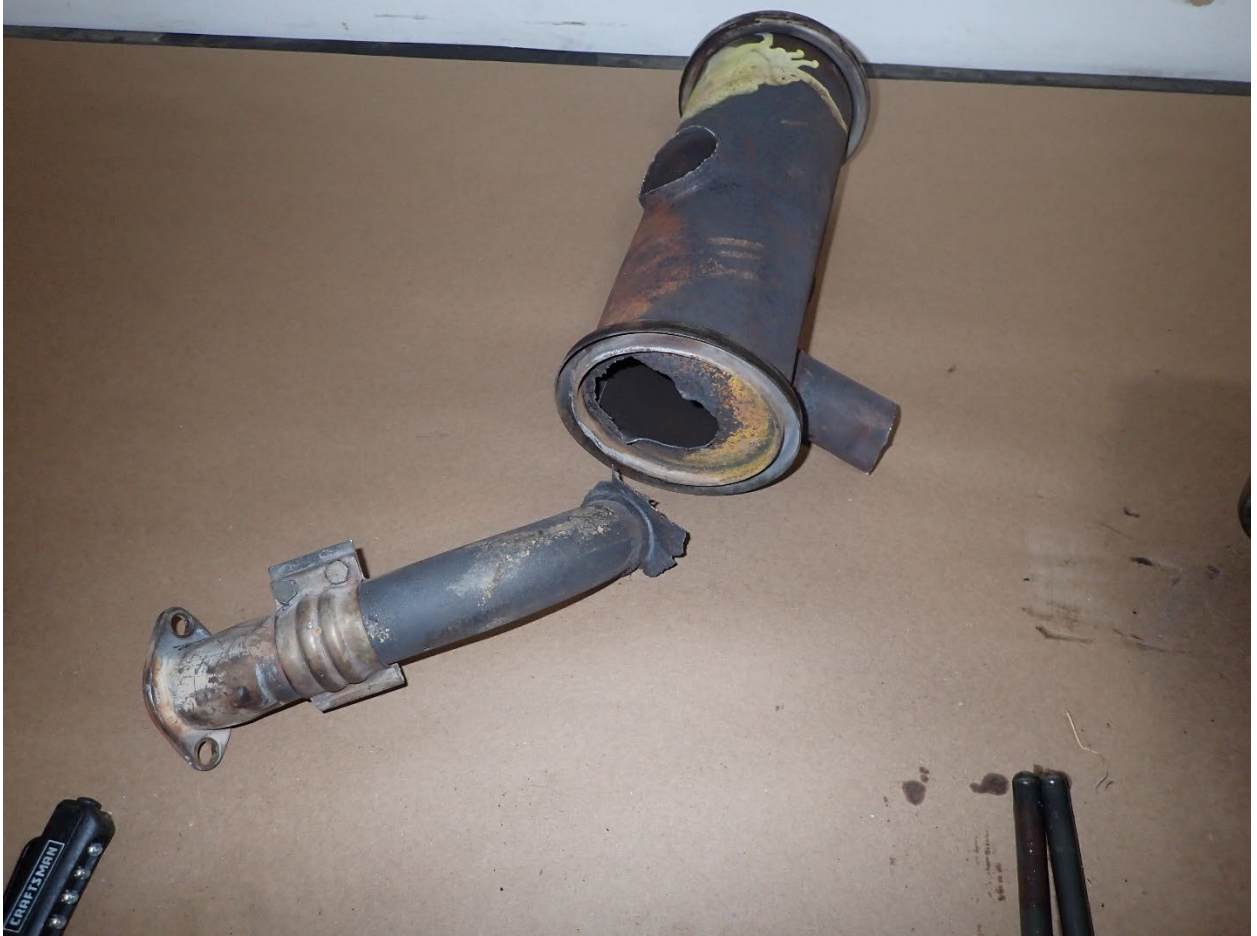
Figure 3 View of the exhaust manifold and muffler.
