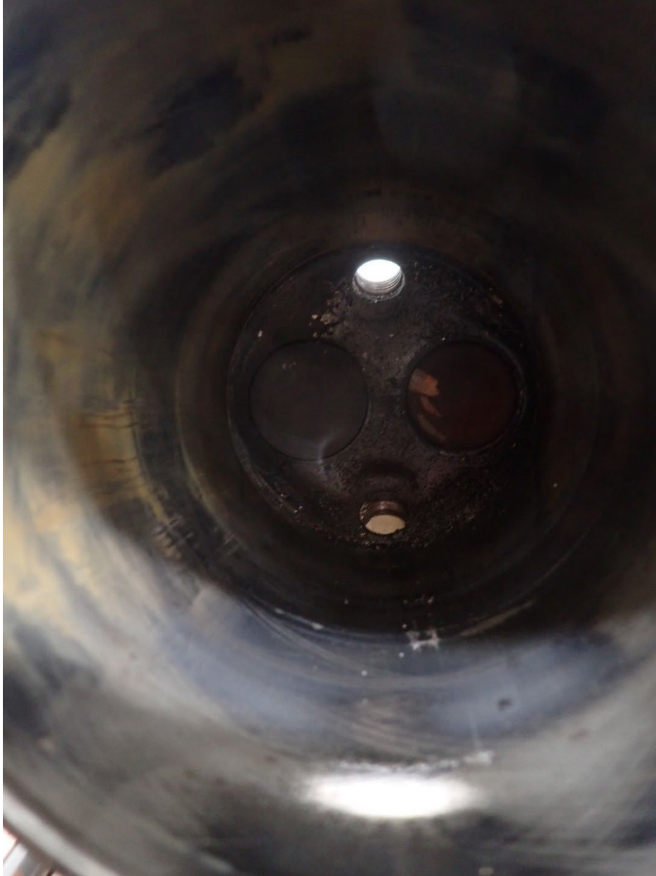
Figure 2 View of the interior of cylinder No. 4, the exhaust valve on the right and remained in the closed position.
