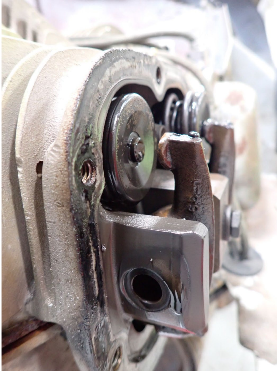
Figure 1 View of cylinder No. 4 exhaust valve.
