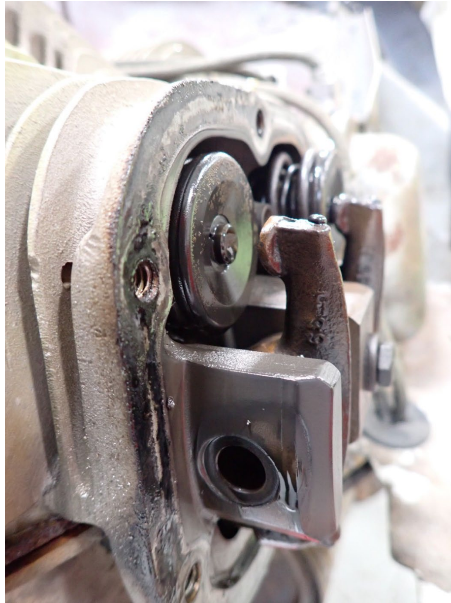
Photo 2 –View of cylinder No. 4 exhaust valve.
