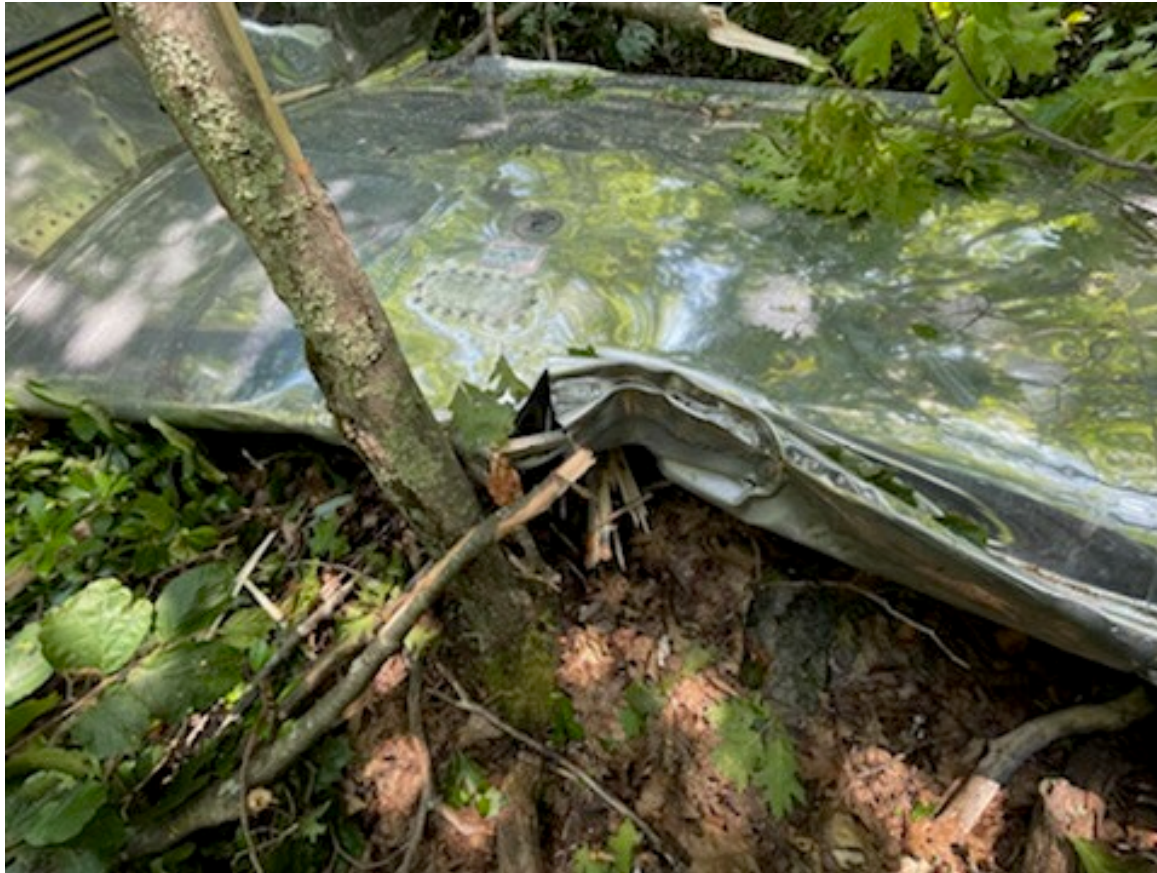
Photograph 3 - Impact damage to left wing (Courtesy of FAA)
