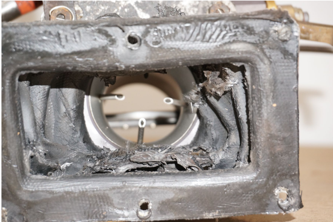
Photograph 6 - Deteriorated fuel injector airbox boot
