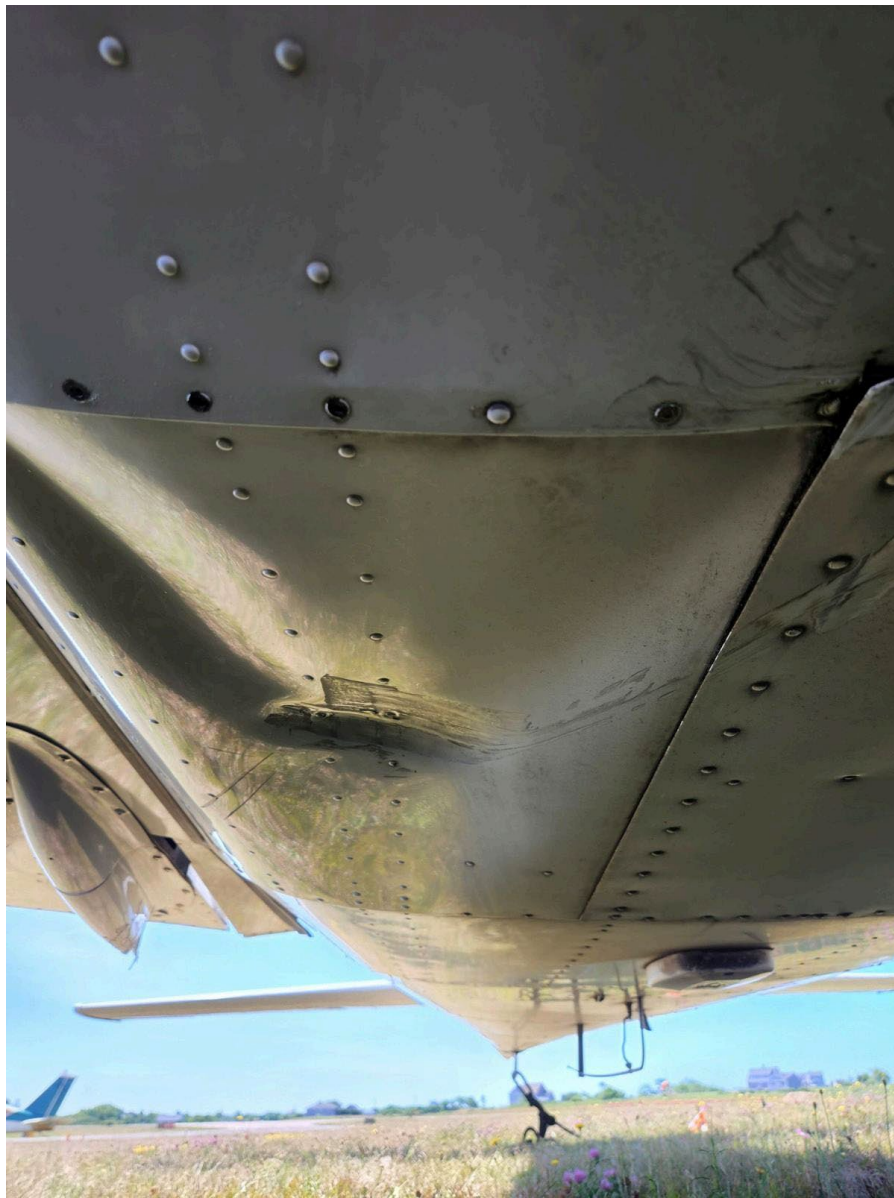
Photo 1: Damage to the airplane's fuselage (Photo Courtesy of FAA)
