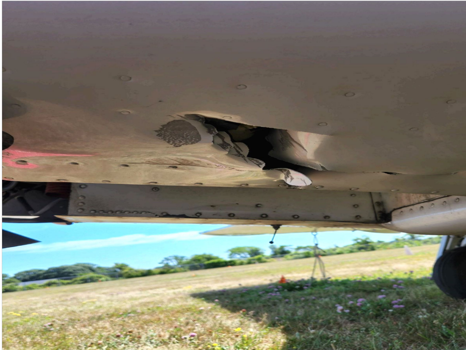
Photo 4: Damage to the airplane's fuselage (Photo Courtesy of FAA)
