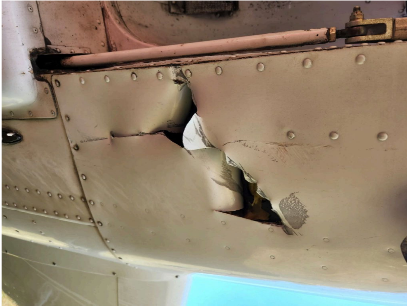
Photo 3: Hole in the airplane fuselage abeam the nose landing gear tunnel wall (Photo Courtesy of FAA)
