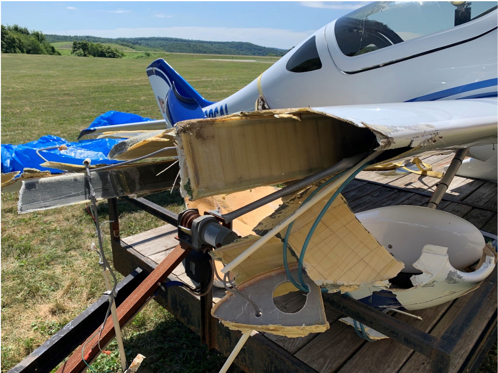
Photo 2 – Right Wing Damage (Photo Courtesy of FAA)
