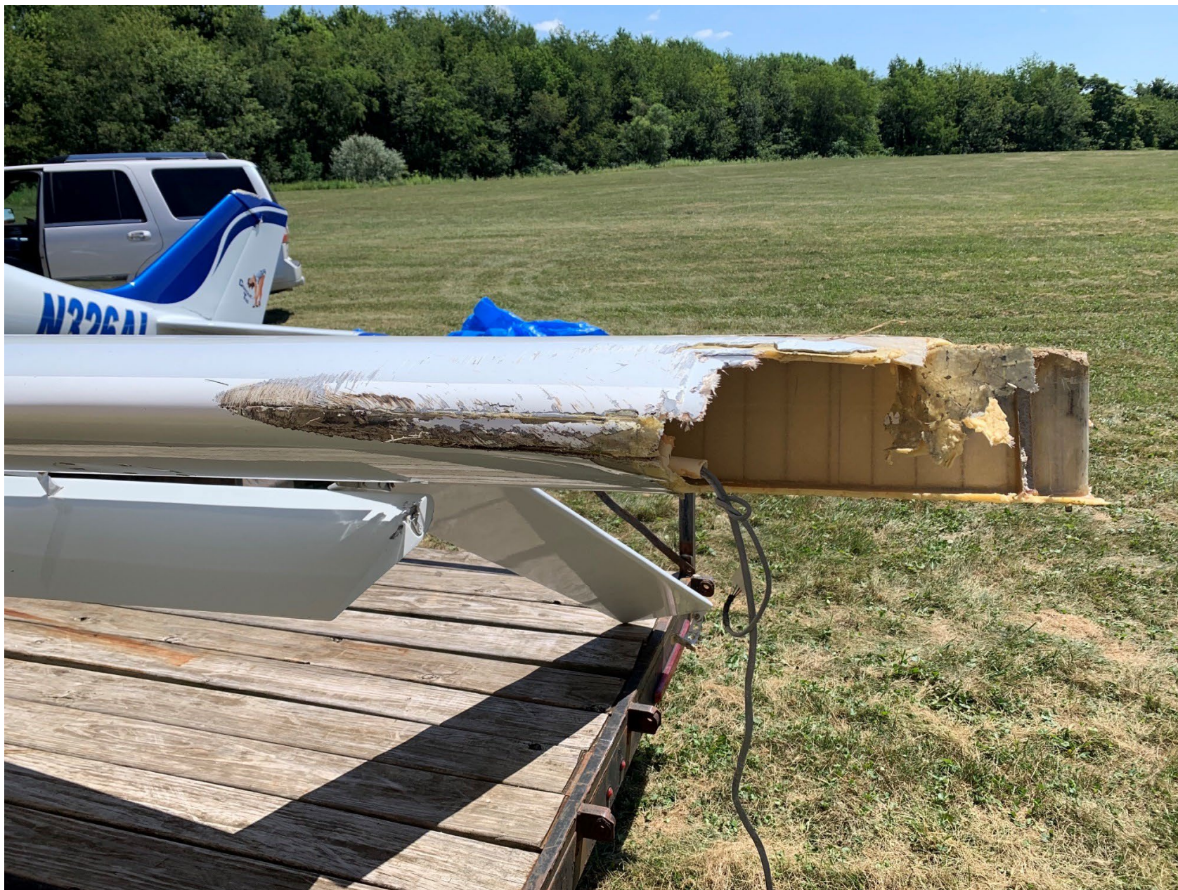
Photo 3 – Left Wing Damage (Photo Courtesy of FAA)
