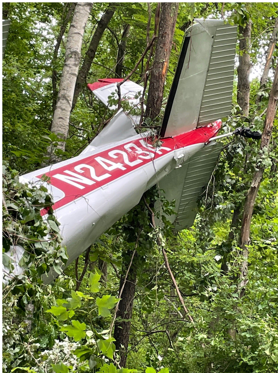
Photo 2 – View of Damage to Tail Section and Vertical Stabilizer (FAA)
